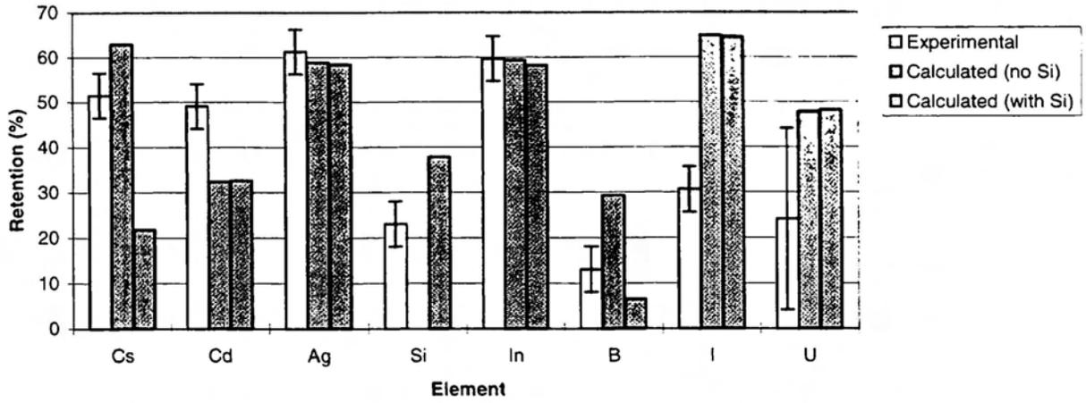
**Figure 2: Comparison Between Experimental and Calculated Retentions of Elements in FALCON FAL ISP-1**
