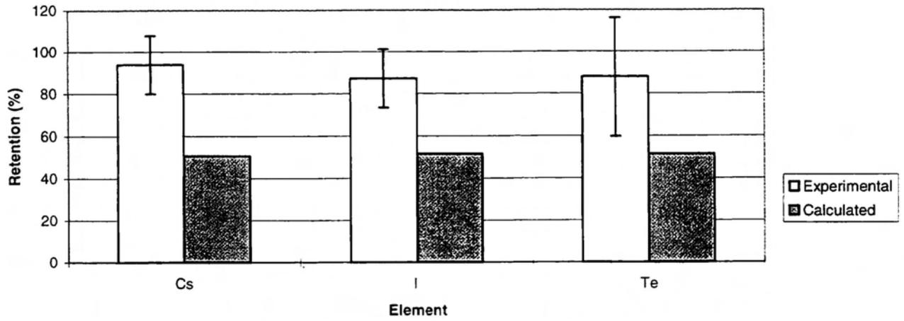
**Figure 1: Comparison Between Experimental and Calculated Retentions for the BTF-104 Experiment**
