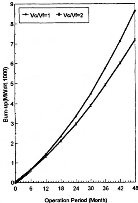
Figure 7. Temporal variation of fissile fuel burn-up in the blankets
