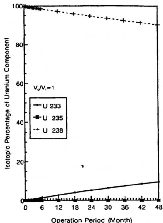
Figure 10. Temporal variation of the percentages of the uranium isotopes in the blankets ( $V_d/V_f = 1$ )
