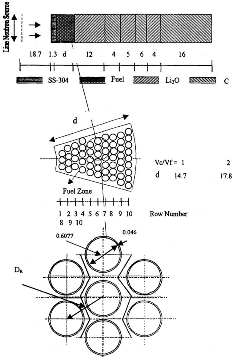
Figure 1. Cross-sectional view of the investigated blanket (dimensions are given in centimetre)
