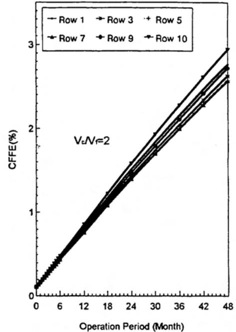
Figure 6. Temporal increase of the fissile fuel enrichment in the blanket ( $V_c/V_f = 2$ )
