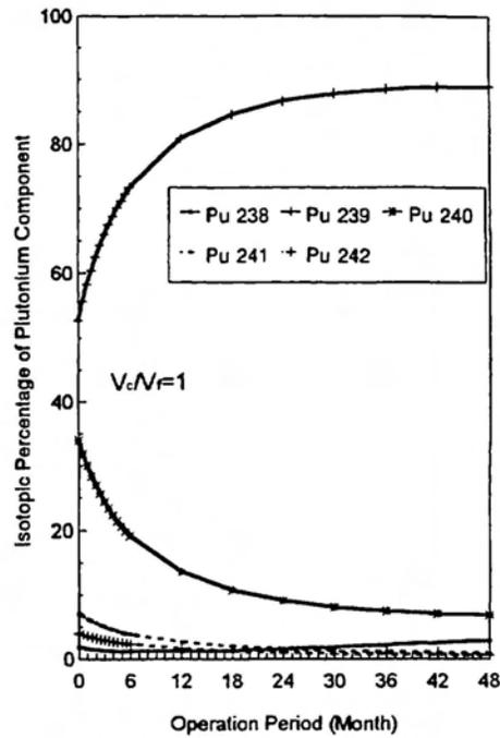
Figure 8. Temporal variation of the percentages of the plutonium isotopes in the blankets ( $V_c/V_f = 1$ )
