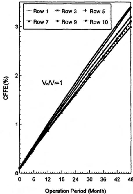
Figure 5. Temporal increase of the fissile fuel enrichment in the blanket ( $V_c/V_f = 1$ )
