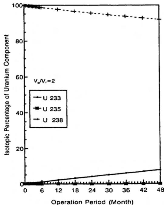
Figure 11. Temporal variation of the percentages of the uranium isotopes in the blankets ( $V_d/V_f = 2$ )
