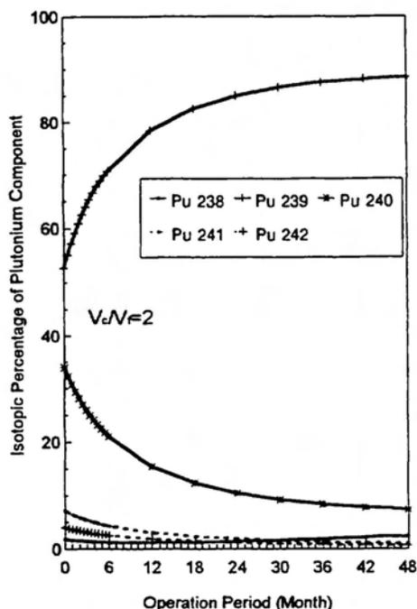
Figure 9. Temporal variation of the percentages of the plutonium isotopes in the blankets ( $V_d/V_f = 2$ )
