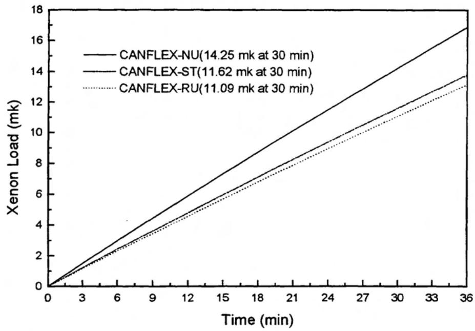
Figure 4. Xenon Transient For 30 Minutes After Reactor Shutdown
