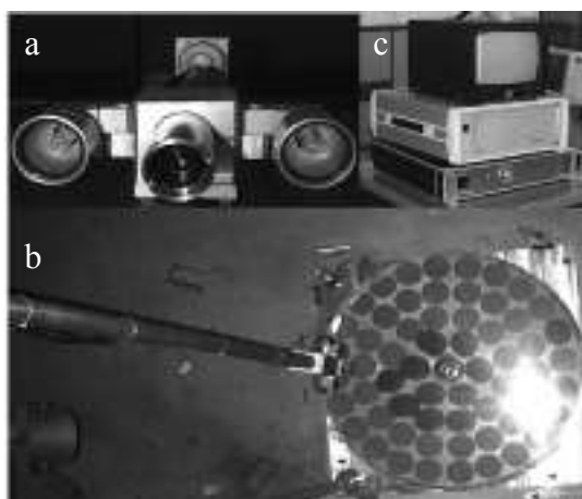
Fig. 7 Photo of SCAI Components (a) Underwater Camera & Light (b) Spent Fuel Basket & Guide Tube (c) Controller & Monitor
