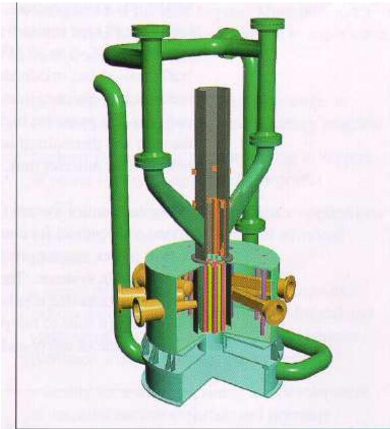
**Figure 1** Multipurpose Applied Physics Lattice Experiment (MAPLE) Reactor
