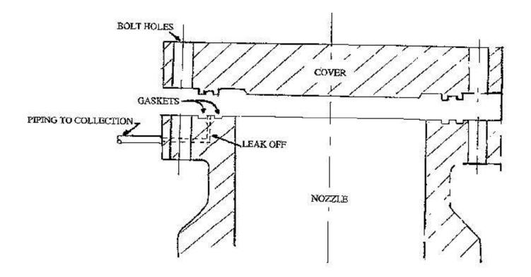
Figure 3: Modified Inspection Port Flange
