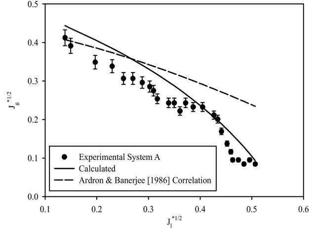
Figure 2. Comparison of predicted and experimental flooding points experiments of Krowlewski [1980].
