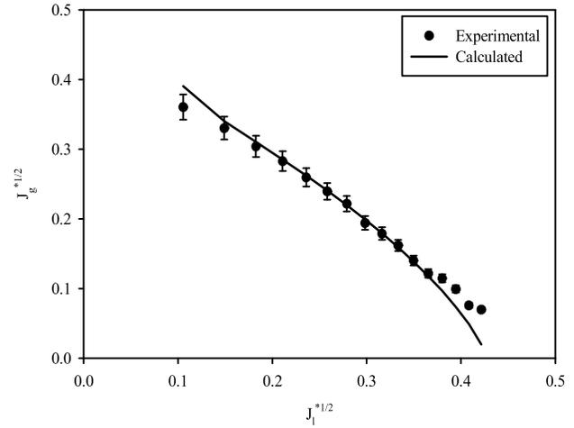
Figure 10. Comparison of predicted and experimental flooding points IGN experiments (Orifice  $\beta=0.66$ ).
