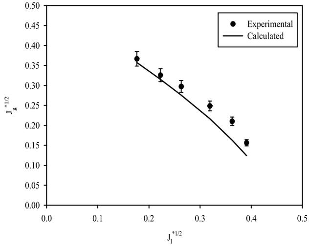
Figure 13. Comparison of predicted and experimental flooding points experiments of Kawaji *et al.* [1993] (Orifice  $\beta=0.67$ )
