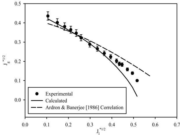
Figure 1. Comparison of predicted and experimental flooding points IGN experiments (no orifice).
