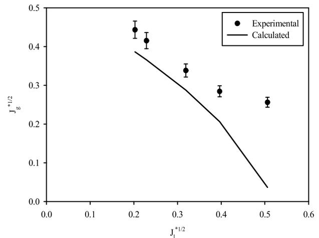
Figure 12. Comparison of predicted and experimental flooding points experiments of Kawaji *et al.* [1993] (Orifice  $\beta=0.865$ ).
