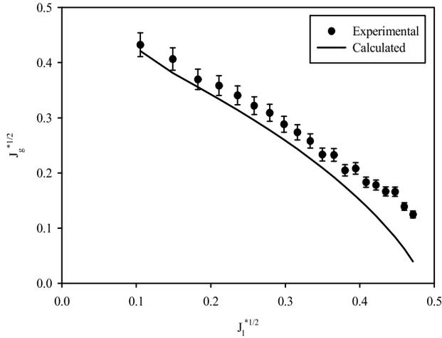
Figure 7. Comparison of predicted and experimental flooding points IGN experiments (Orifice  $\beta=0.83$ ).
