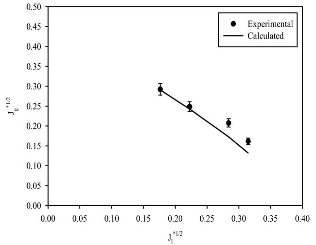
Figure 14. Comparison of predicted and experimental flooding points experiments of Kawaji *et al.* [1993] (Orifice  $\beta=0.55$ )
