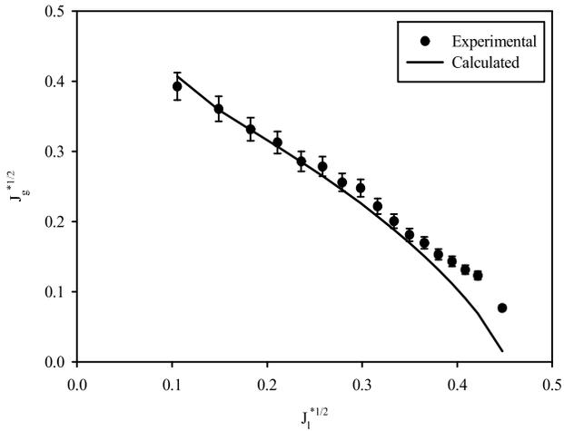
Figure 9. Comparison of predicted and experimental flooding points IGN experiments (Orifice  $\beta=0.72$ ).
