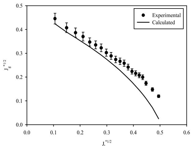
Figure 6. Comparison of predicted and experimental flooding points IGN experiments (Orifice  $\beta=0.90$ ).
