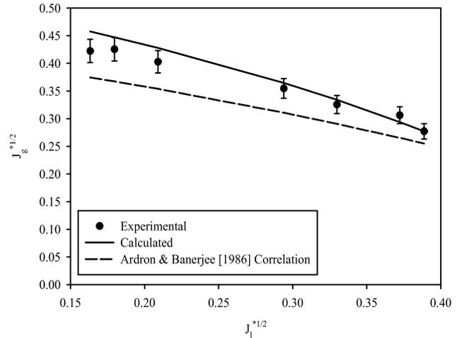
Figure 4. Comparison of predicted and experimental flooding points experiments of Siddiqui *et al.* [1986].
