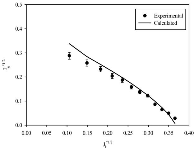
Figure 11. Comparison of predicted and experimental flooding points IGN experiments (Orifice  $\beta=0.55$ ).
