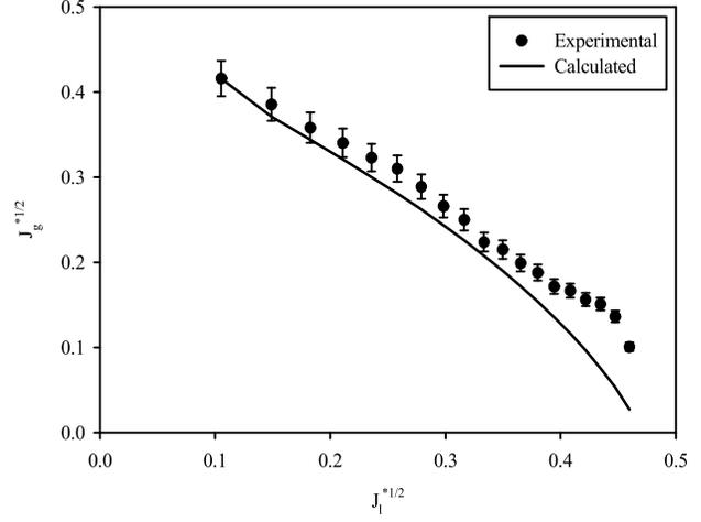
Figure 8. Comparison of predicted and experimental flooding points IGN experiments (Orifice  $\beta=0.77$ ).
