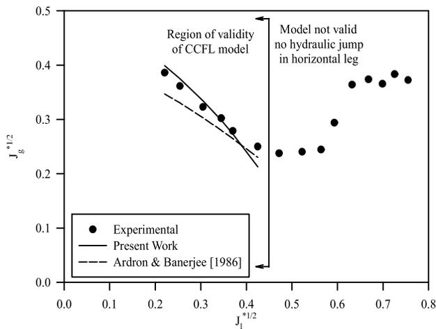
Figure 5. Comparison of predicted and experimental flooding points experiments of Kawaji *et al.* [1991]
