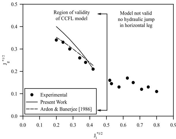
Figure 3. Comparison of predicted and experimental flooding points experiments of Wan & Krishnan [1986].
