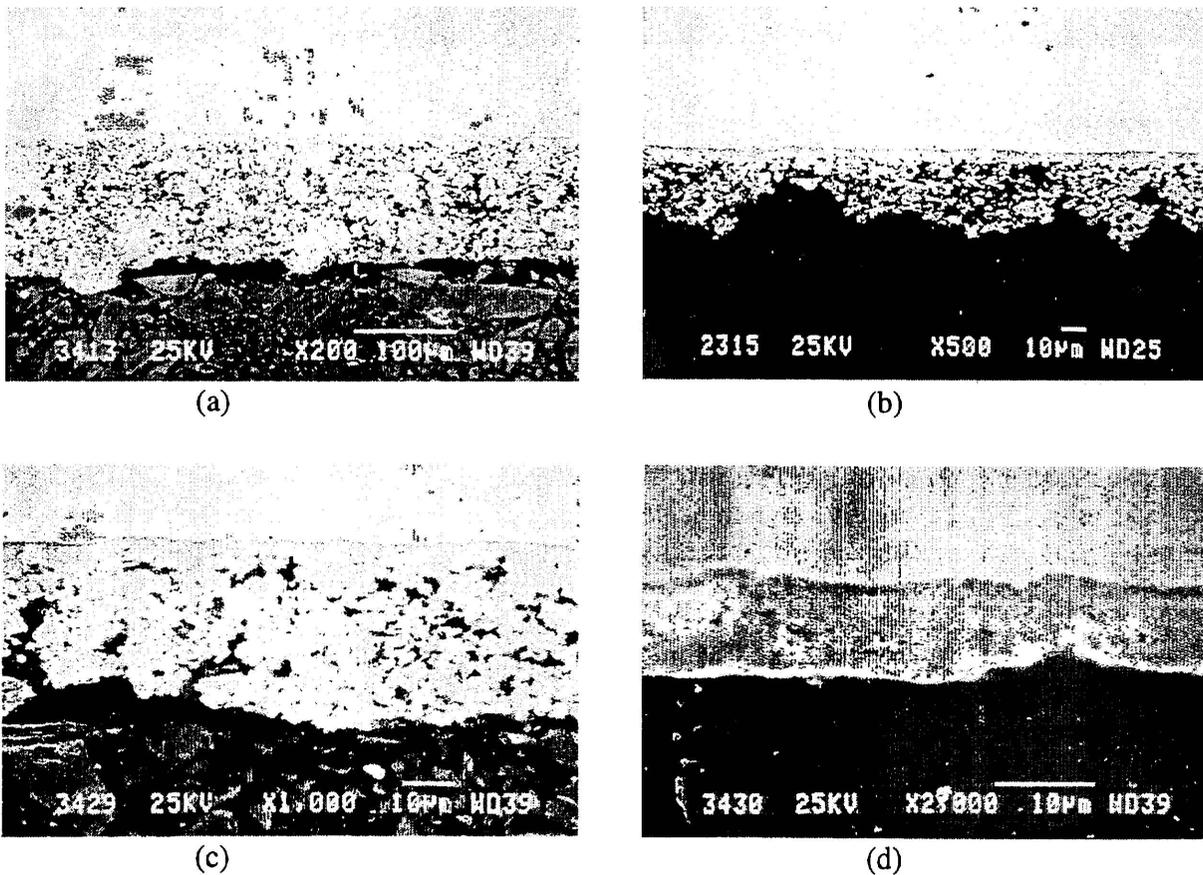
Figure 4: Examples of SEM micrograph of metallographic cross sections showing the thickness profile of the tube deposits (a) before removal, (b) after chemical removal, (c) after mechanical removal (first step), and (d) after the mechanical removal (second step).
