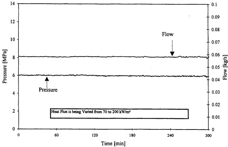
Figure 2: Stability of the experimental conditions during the tests.
