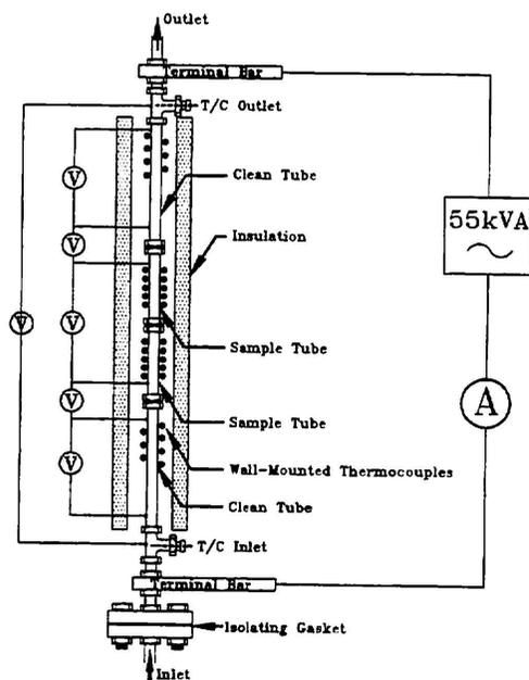
Figure 1: The experimental test section.
