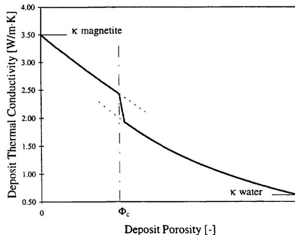
Figure 5: Schematic representation of the dependence of the thermal conductivity of a magnetite-water composite on porosity (volume fraction of water).  $\Phi_c$  is the percolation porosity of the structure at which the particles of magnetite become effectively separated from each other.
