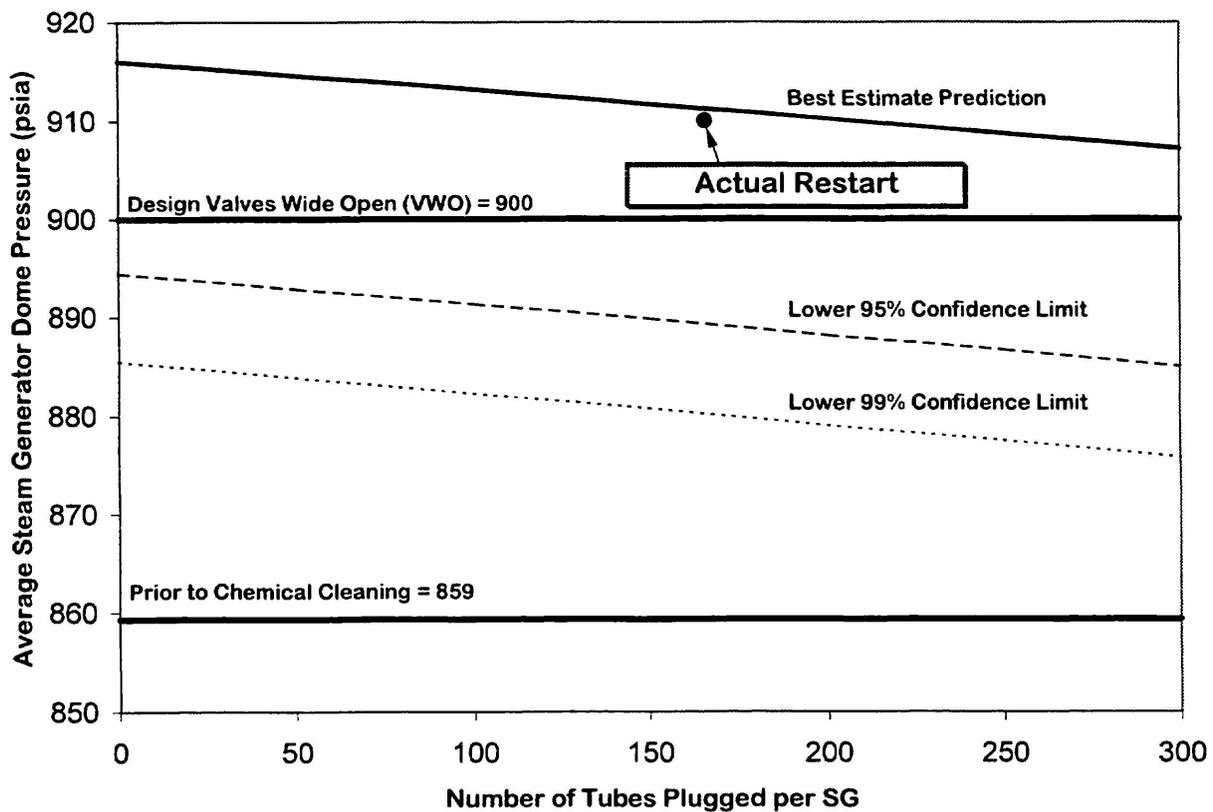
Figure 7. Predicted Steam Pressure After Chemical Cleaning at San Onofre 2
