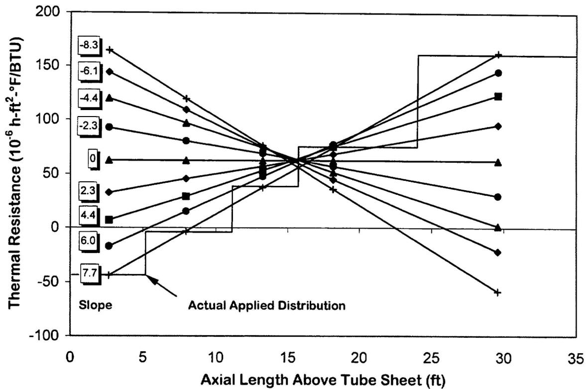
Figure 8. Linear Variations of Fouling Factor Applied to ATHOS Model ( $60 \cdot 10^{-6}$  Avg)
