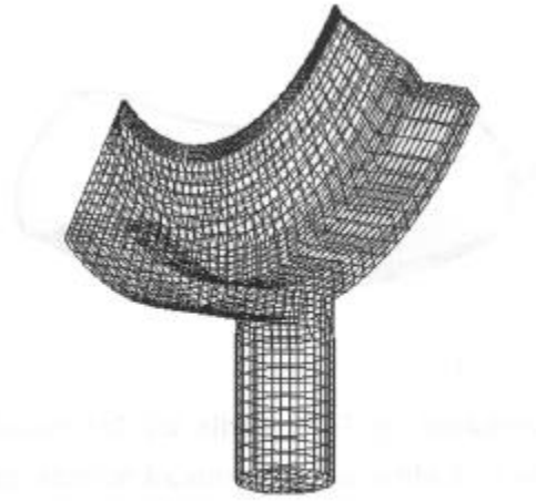
Fig. 2 Mesh grid of HPTB extraction line
