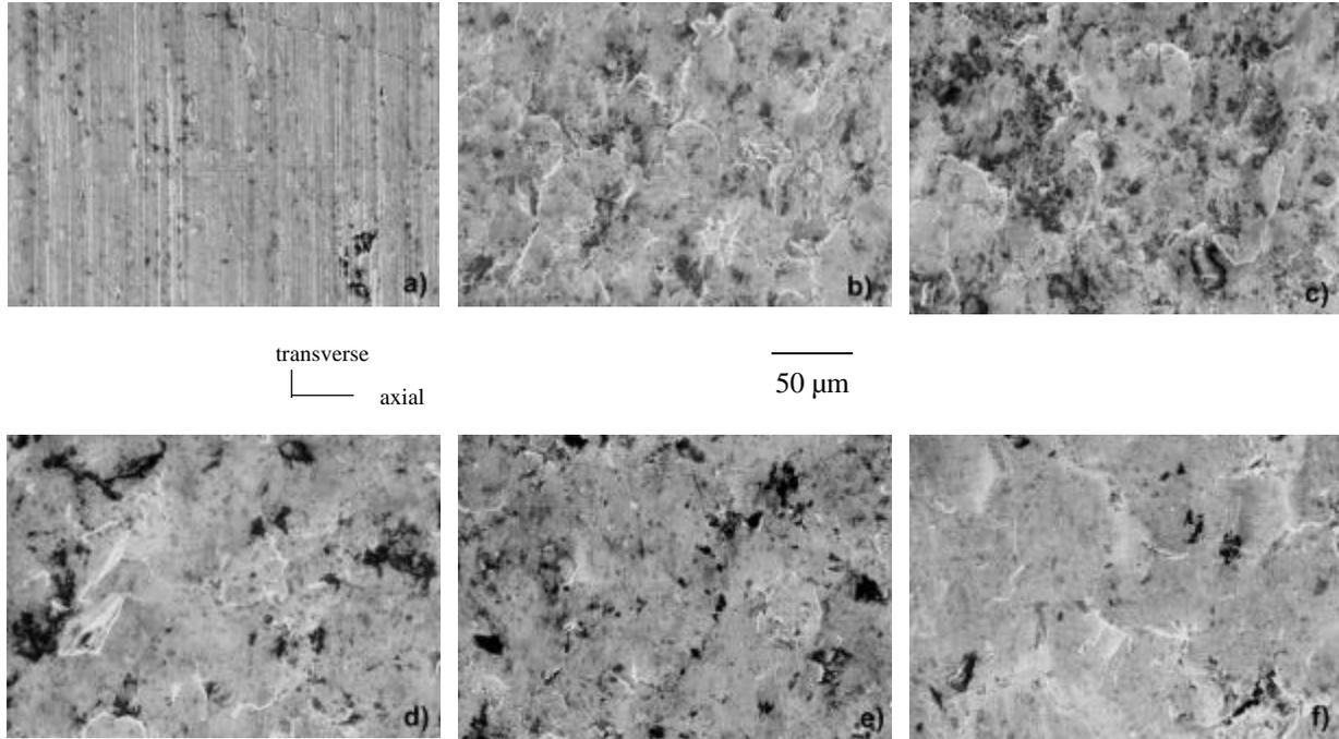
**Figure 2.** Comparison of surface topology of as-received and variously-peened tubes:
