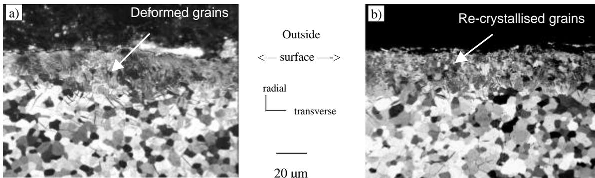
**Figure 6.** Micrographs Showing (A) As-Peened Tube with Deformed Grains Below the Peened Surface, And (B) Peened and Stress-Relieved Tube with Recrystallised Grains in the Peened Region.
