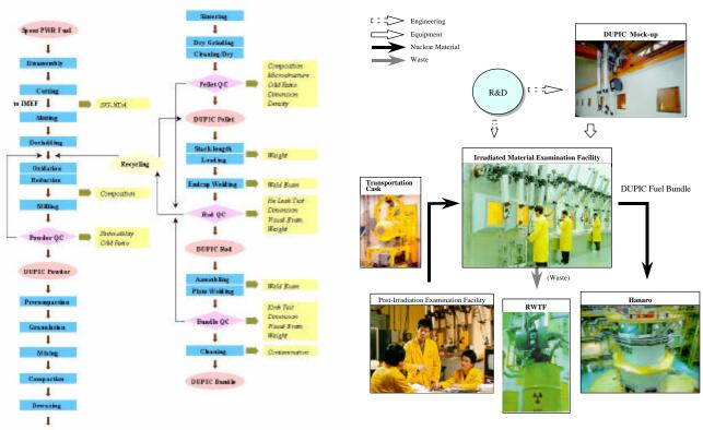
Figure 1. DUPIC Fuel Fabrication Processes
