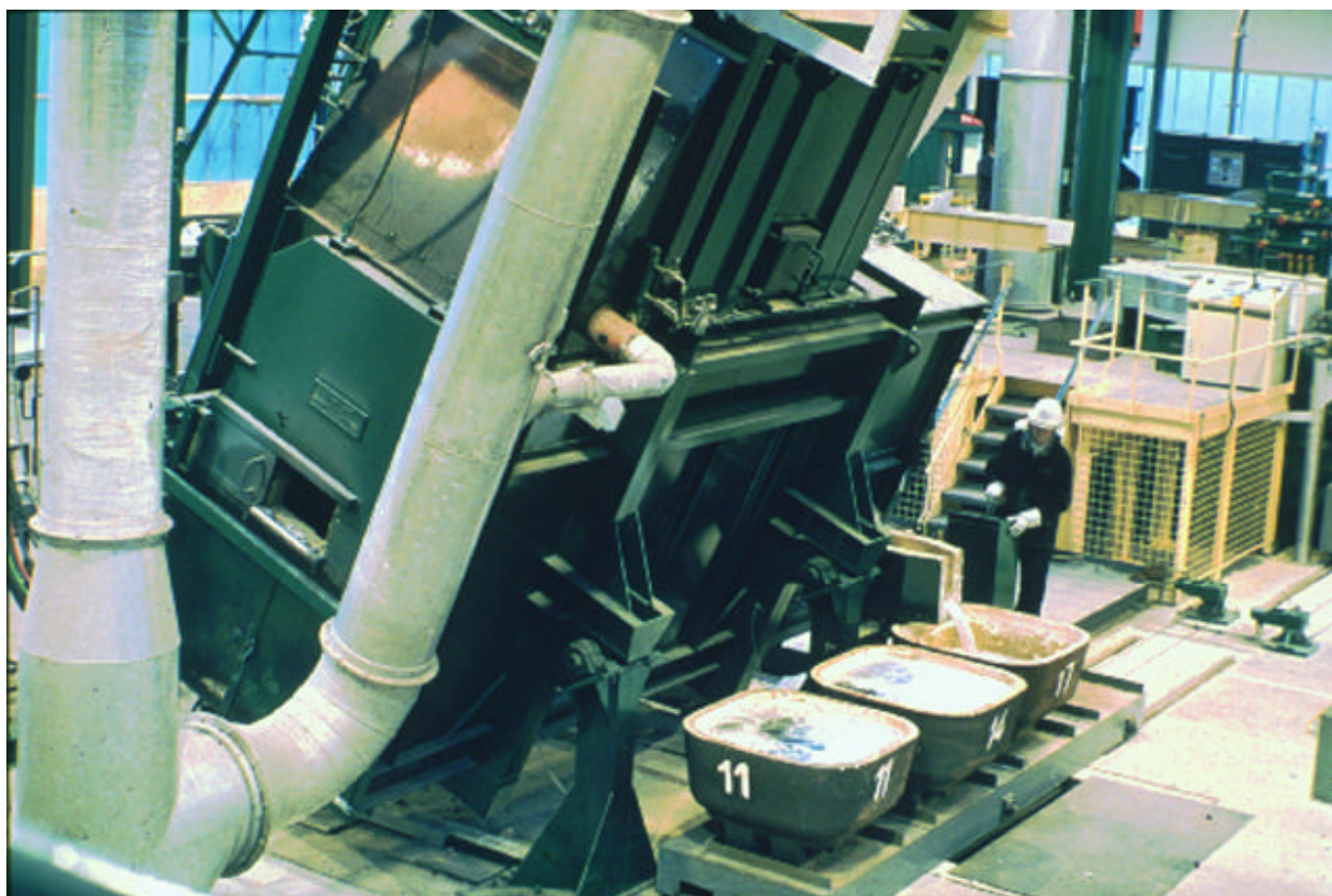
Figure 7 The melter has been used to process a range of contaminated metals.
