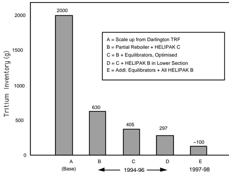
**Fig. 2 Isotope Separation System - Inventory Reduction in Final Column (based on throughput of 200Pa.m<sup>3</sup>/s.)**
