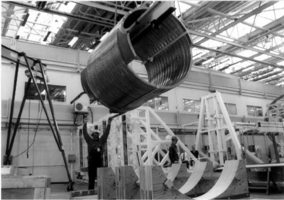
**Figure 2** Inner layer of the inner module of the CS Model Coil
