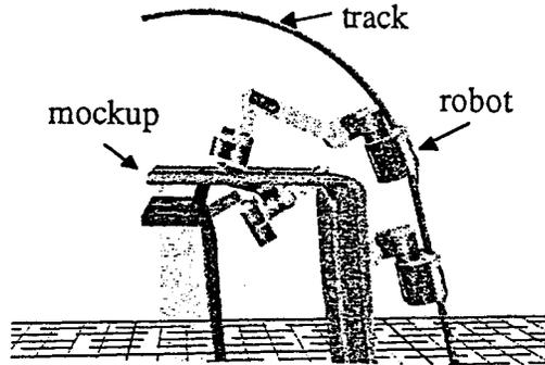
**Figure 4** Computer simulation showing robotic welding system for vacuum vessel mockup
