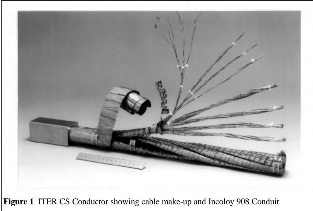
**Figure 1** ITER CS Conductor showing cable make-up and Incoloy 908 Conduit
