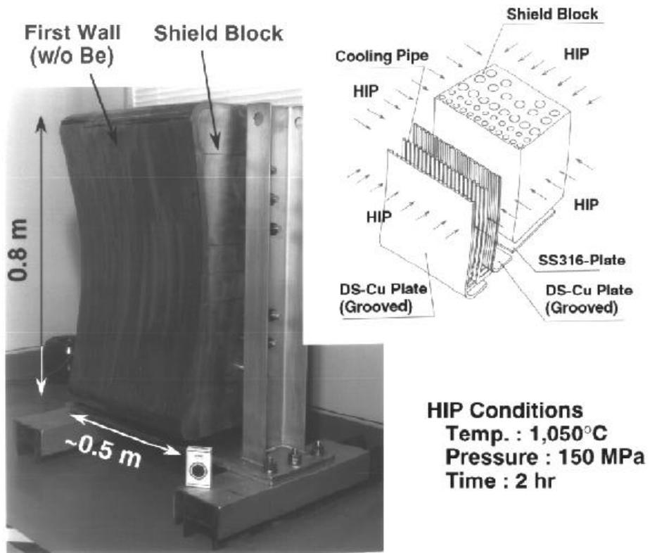
**Figure 5** A half-scale module successfully fabricated by one-step Hot Isostatic Pressing bonding technique.
