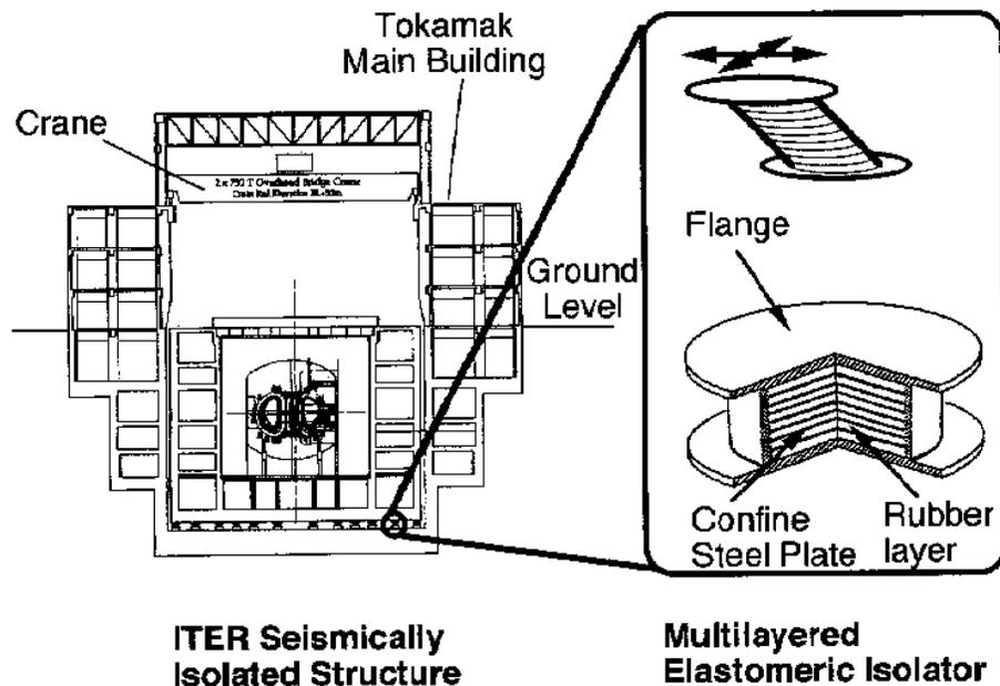
**Figure 10** Seismic design by supporting Tokamak pit base using multilayered elastomeric isolators.
