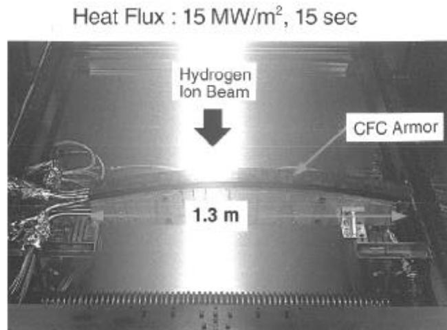
**Figure 6** Full length 1.3 m long divertor element under ion beam irradiation test.
