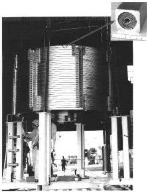
**Figure 3** First layer after the heat treatment for the CS model coil. The conductor is made of twisted 1000 Nb<sub>3</sub>Sn strands inserted and compacted in a high nickel steel (Incoloy) jacket
