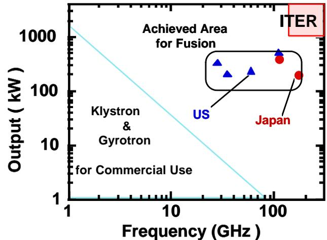
Figure 8 A 170 GHz Gyrotron under development for heating and current drive aims by far the commercially available performance.
