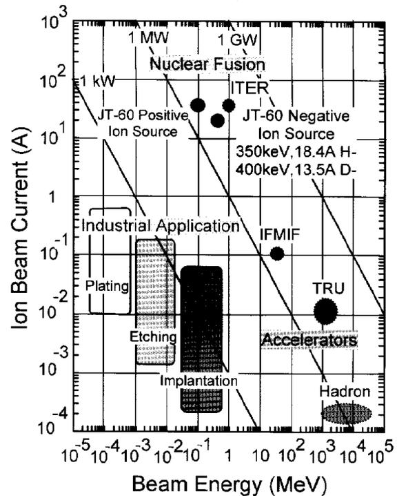
Figure 7 Output power of ion beam for fusion and various applications and requirement. Ion beam for fusion is leading multi-megawatts source development.
