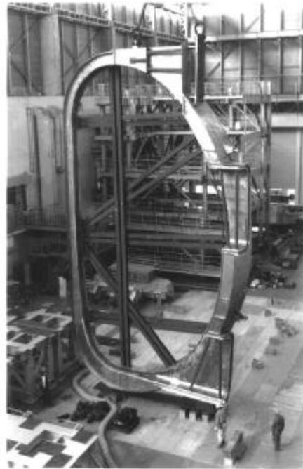
**Figure 4** Vacuum vessel full-scale sector model before in-situ welding along the poloidal contour.
