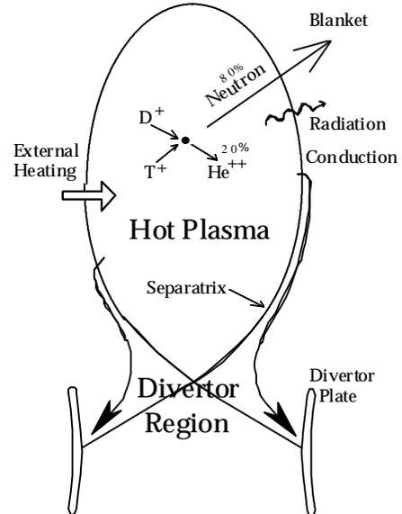
Figure 1 Heat Flow Schematic of Reactor
