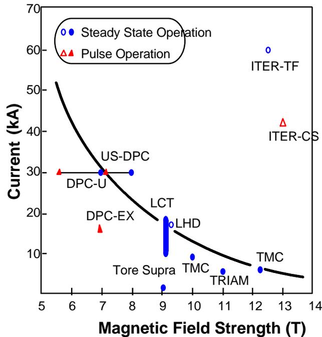
**Figure 2** Characteristics of the superconducting conductors for ITER compared with those for other devices or coils.
