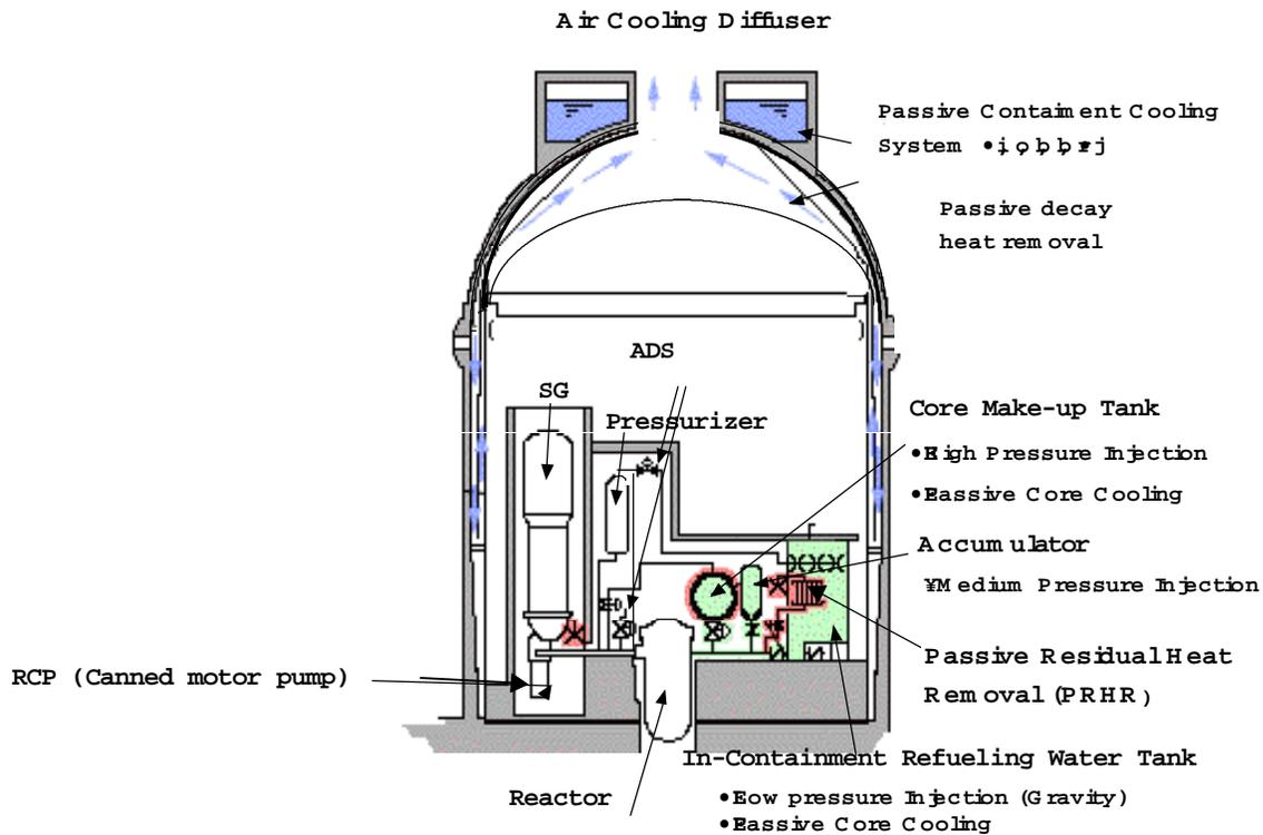
Figure 3: SPWR plant concept
