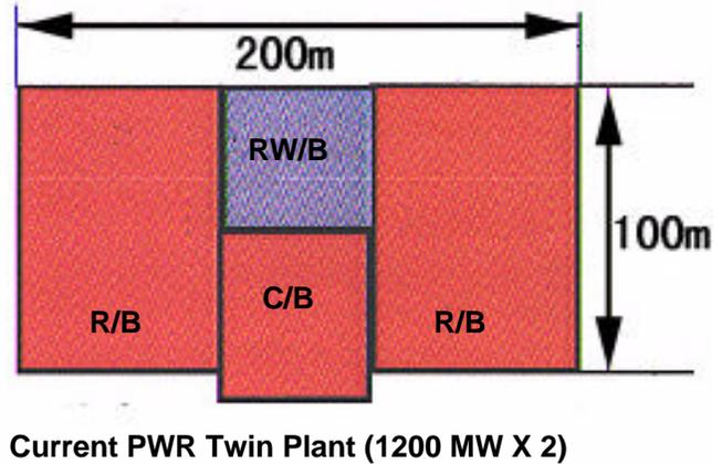
Figure 4: The R/B footprint comparison between SPWR and current plant
