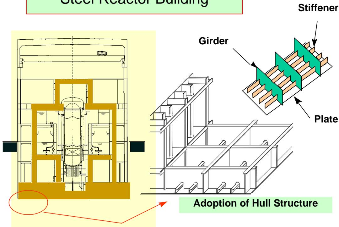
Figure 10 : Hull structure adoption to JSBWR plant
