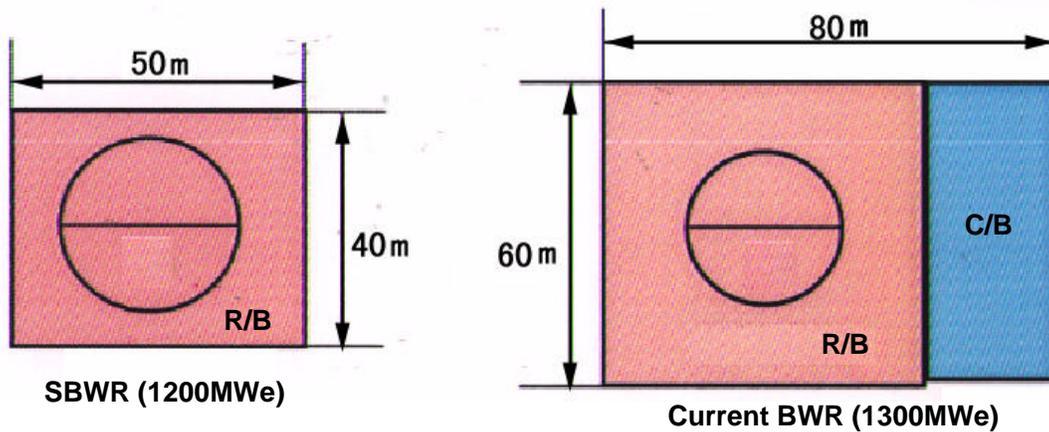
**Figure 7: The R/B footprint comparison between JSBWR and current plant**
