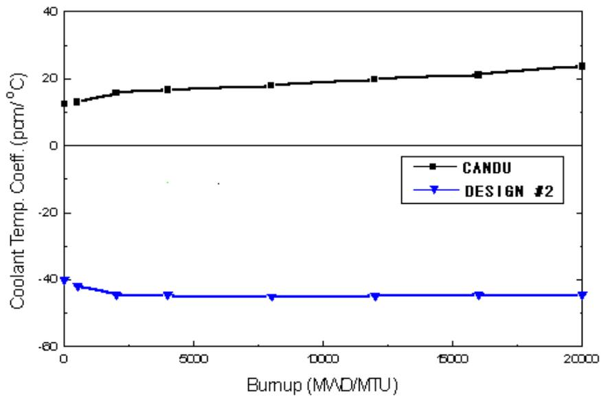
Figure 6. CTC of Reactor Module Design #2
