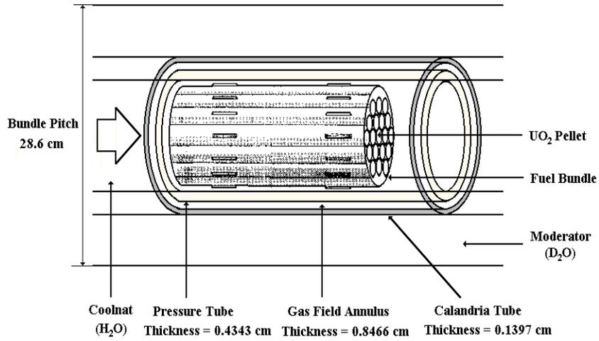
Figure 1. Unit Module of CANDU reactor channels
