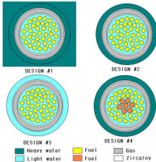
Figure 2. Reactor Modules of Fuel, Coolant, and Moderator
