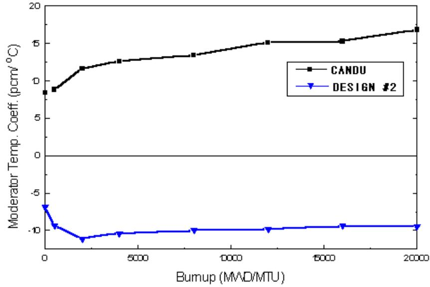
Figure 7. MTC of Reactor Module Design #2
