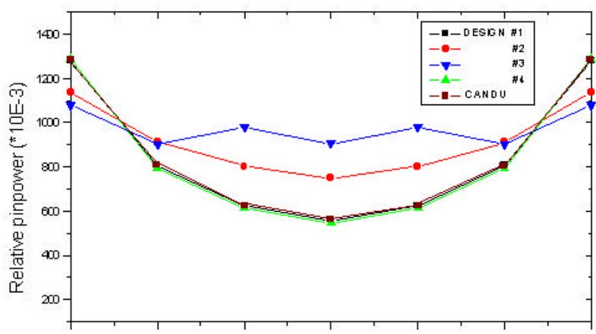
Figure 4. Relative Pin Power Distribution in Fuel Bundles
