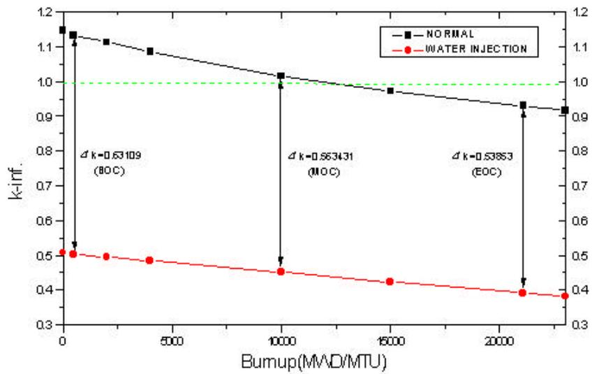
Figure 5. Reactivity Change of Reactor Module for the Emergency Water Injection
