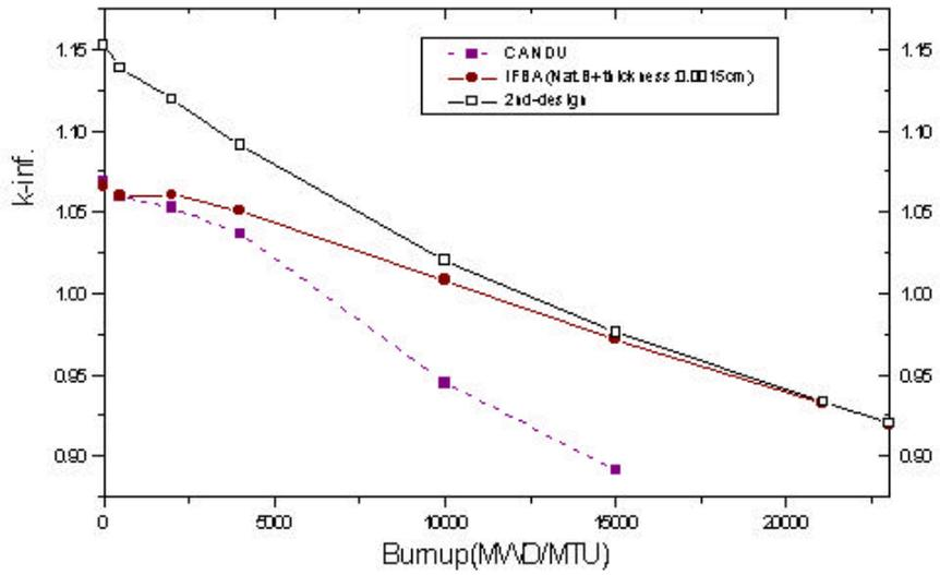
Figure 8. Excess Reactivity Change with IFBA in Design #2
