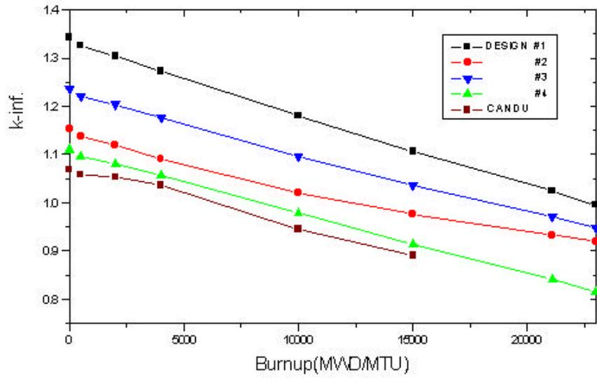
Figure 3. K-infinite Change of Reactor Modules vs. Fuel Burnup
