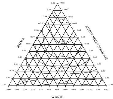
**Figure 12** Contours of irradiation resistance (added impurities)
