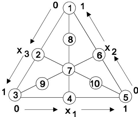
**Figure 1** The simplex-centroid design including 3 interior points
