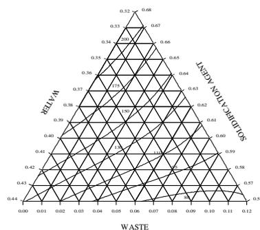
**Figure 7** Contours of water-immersion resistance (no added impurities)
