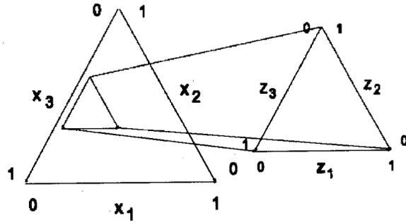
**Figure 2** Transformation of a sub-region of the original simplex to a full L-pseudocomponent simplex
