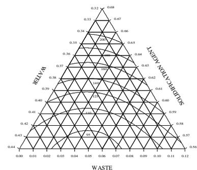
**Figure 8** Contours of water-immersion resistance (added impurities)
