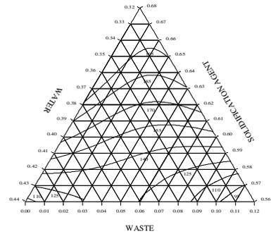
**Figure 11** Contours of irradiation resistance (no added impurities)
