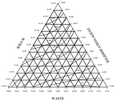
**Figure 9** Contours of thermal cycling resistance (no added impurities)
