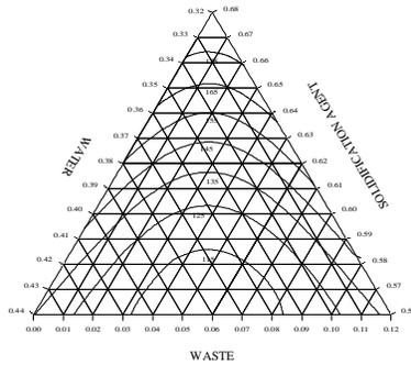
**Figure 10** Contours of thermal cycling resistance (added impurities)
