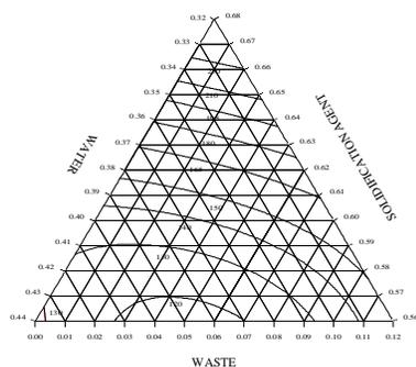
**Figure 6** Contours of compressive strength (added impurities)
