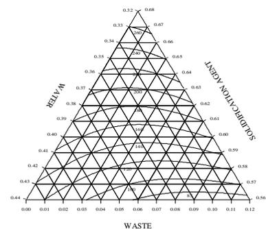
**Figure 5** Contours of compressive strength (no added impurities)
