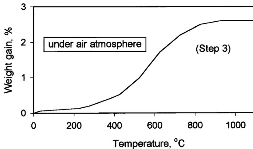
Fig. 3. TG analyses of ruthenium trapped on an yttria filter under hydrogen atmosphere (Step 2) and under air atmosphere (Step 3).
