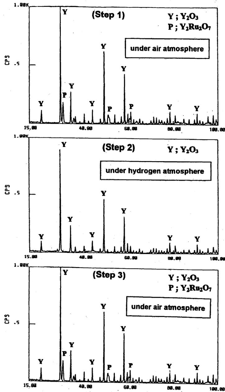
Fig. 2. XRD analyses of ruthenium trapped on an yttria filter under air atmosphere(Step 1), under hydrogen atmosphere (Step 2) and under air atmosphere((Step 3).
