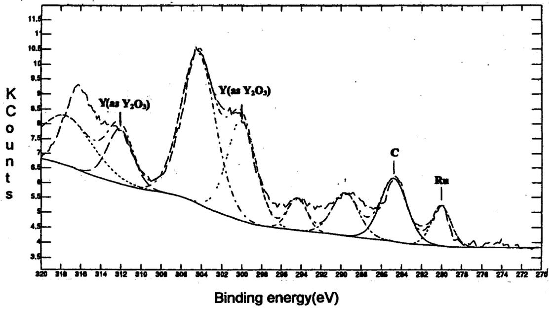
Fig. 4. X-ray photoelectron spectrum of reduced sample(Step 2).
