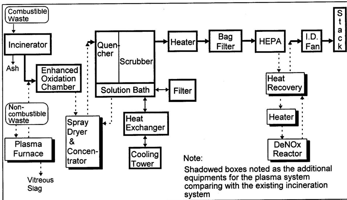
**Figure 3** Flow diagram of a plasma processing system
