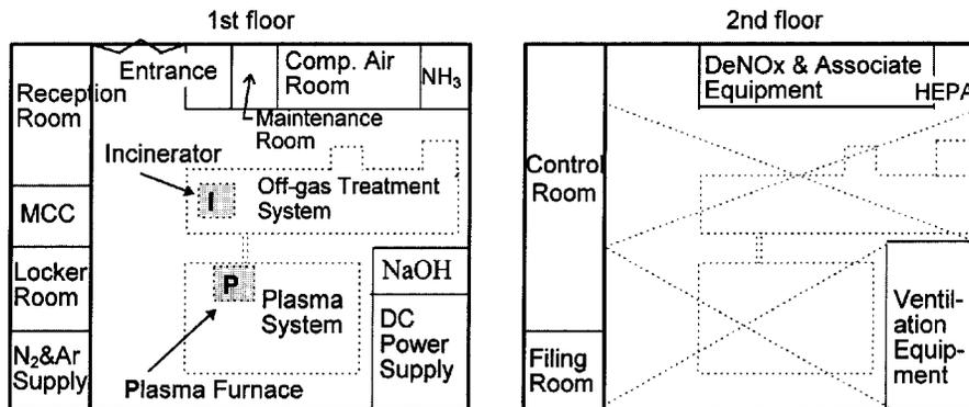
**Figure 2** The layout drawing of a plasma processing facility
