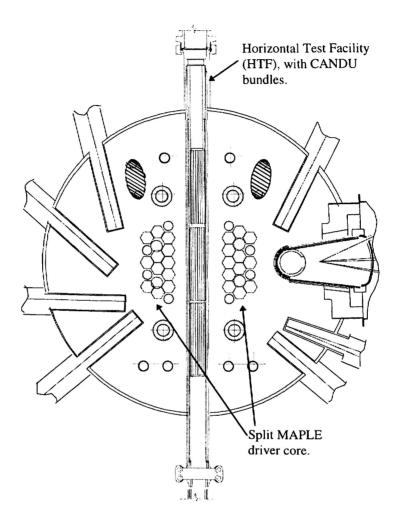
Figure 1. Plan view of proposed IRF, shown with three CANDU test bundles in one of three horizontal test channels (channels are stacked vertically between driver-core halves).
