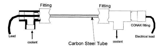
Figure 3 A schematic diagram of the tube version carbon steel thinning rate monitor
