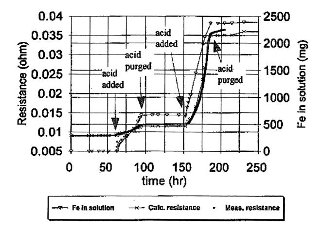
Figure 5 Comparisons between the electrical signal calculated based on the amount of iron lost into the solution and the measured electrical signal at 25 °C.
