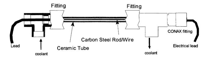
Figure 2 A schematic diagram of the rod and wire version carbon steel thinning rate monitor
