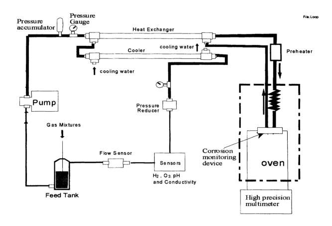
Figure 1 A schematic diagram of the high temperature loop
