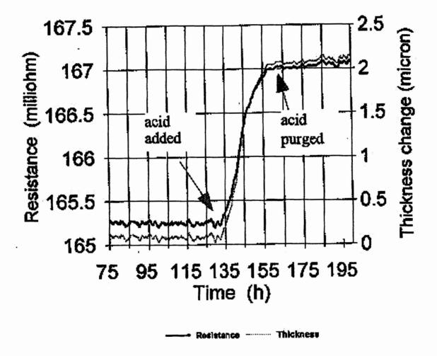
Figure 10 The response of the corrosion rate monitor to the addition of H<sub>2</sub>SO<sub>4</sub> into the LiOH solution, using a carbon steel wire as the sensing element.
