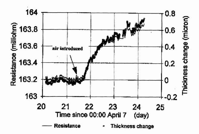
Figure 6 The response of the corrosion rate monitor to the addition of air into the LiOH solution at 310°C, using a carbon steel wire as the sensing element.
