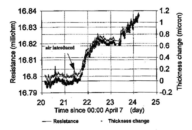
Figure 7 The response of the corrosion rate monitor using a carbon steel rod (A106B) as the sensing element to the addition of oxygen into the LiOH solution at 310°C. After air addition, pH changed from 9.5 to 8 and dissolved O<sub>2</sub> changed from 35 ppb to >350 ppb; Fluid velocity: 4.9 m/s; Diameter of the wire: 0.75 mm.
