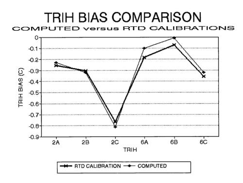
The biases from the independent methods closely agree. The one-sigma deviation of their differences is  $\pm 0.04$  °C. There appears to be little if any systematic differences. These results also indicate that the biases do not change significantly over time since these tests were conducted about three months apart.
