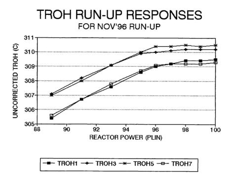
It is apparent from the "flattening" of the TROH responses to increasing power that all four ROHs entered saturation before full power. Below is a table of the TROH bias computations:
