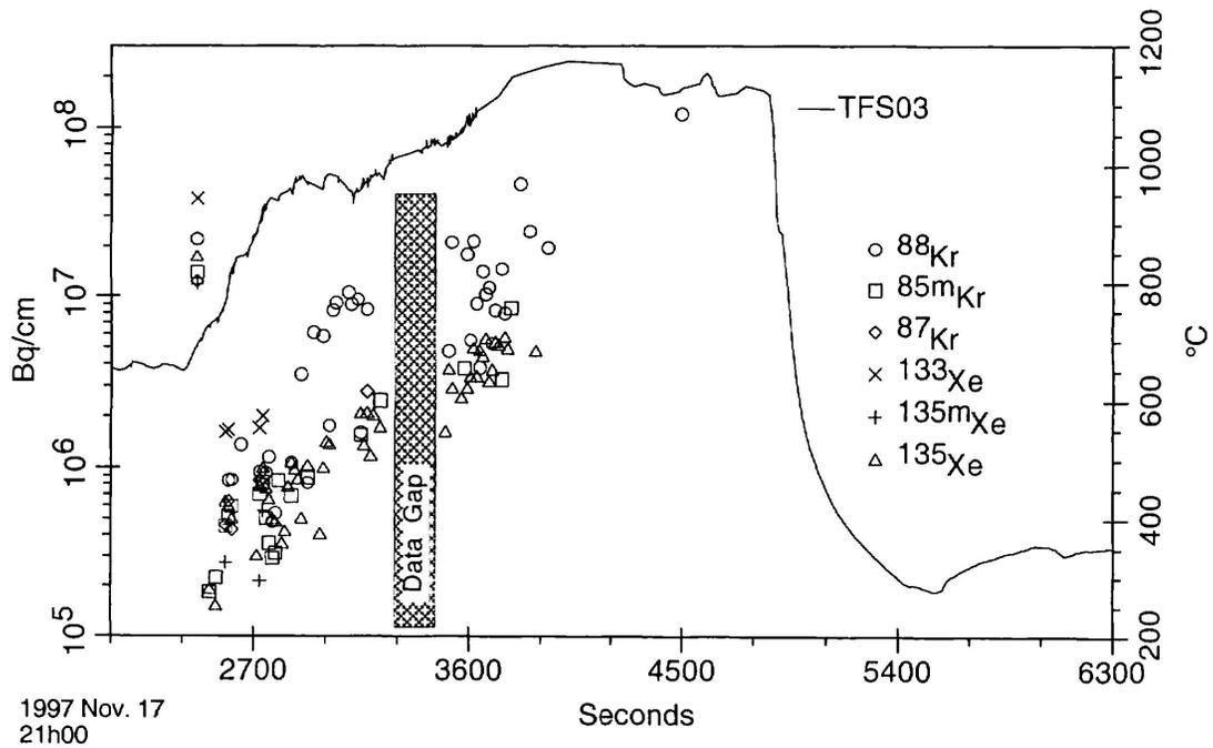
Figure 10: Noble Gas Activity at NW4 and Sheath Thermocouple Temperature
