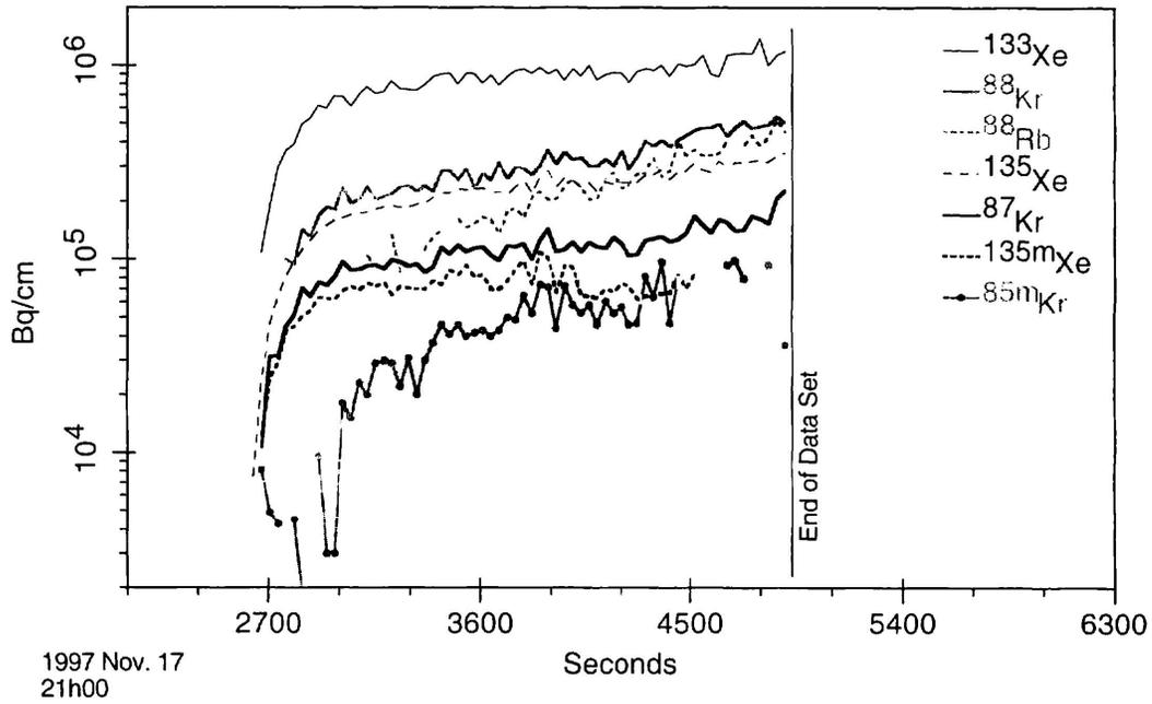
Figure 13: Noble Gas Activity in Liquid Side-Stream from Blowdown Tank
