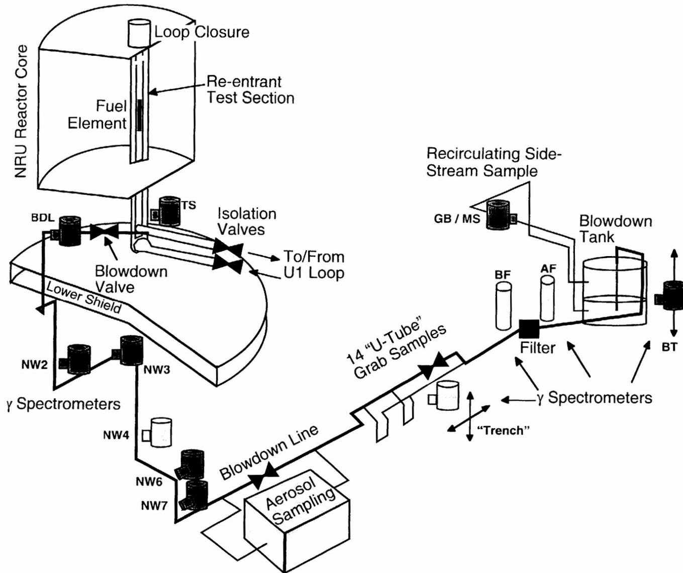
Figure 2: NRU Reactor and BTF
