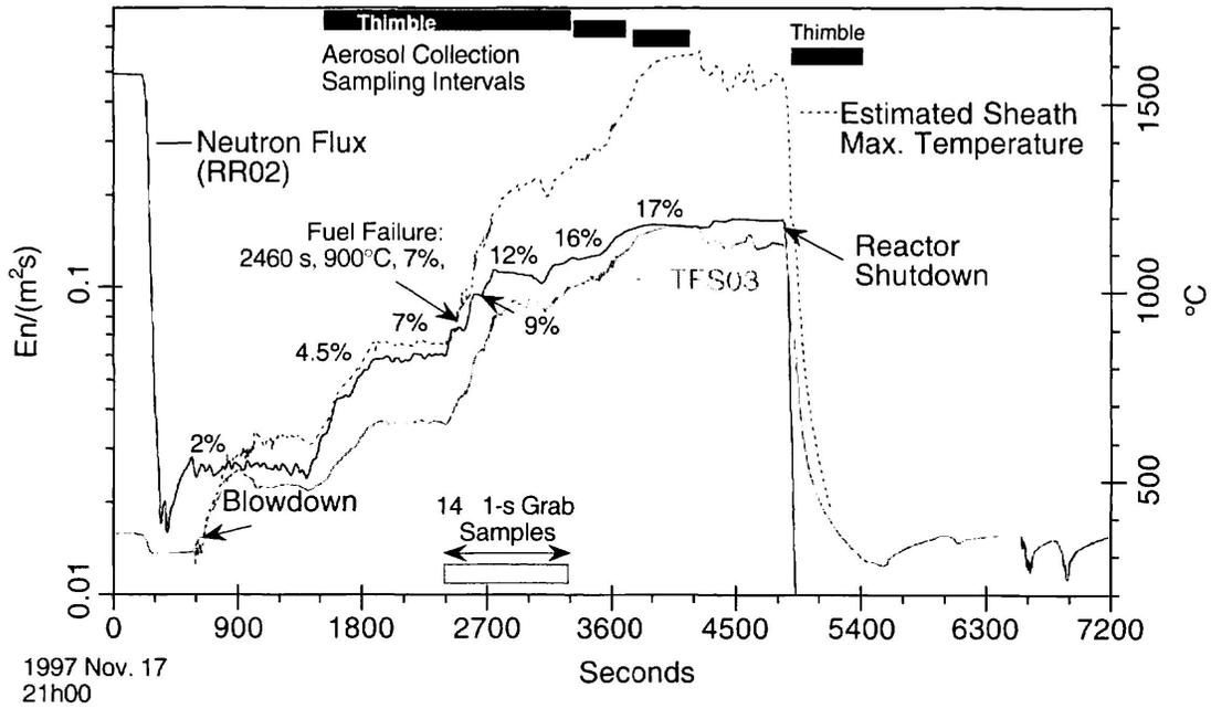
Figure 3: *Neutron Flux and Sheath Thermocouple Temperature*
