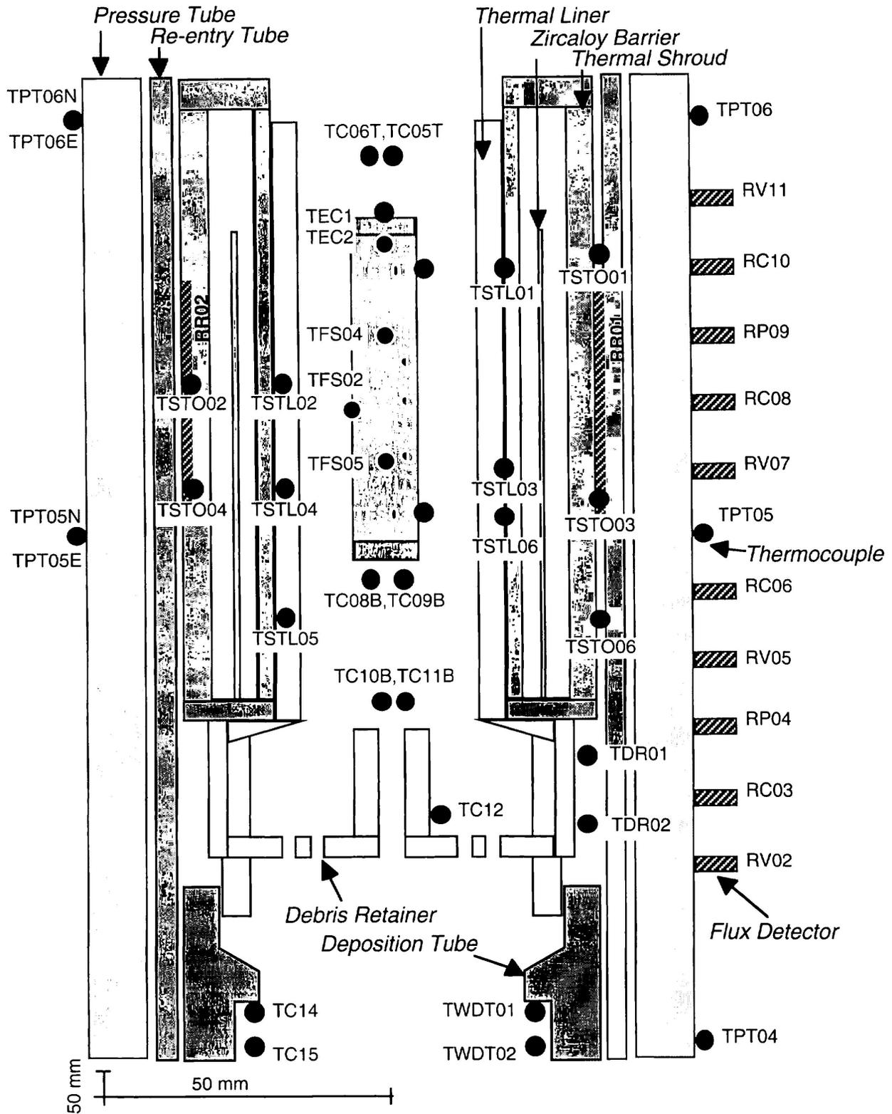
Figure 1: Cross-Sectional View of BTF-105B Fuel Assembly and its Instrumentation
