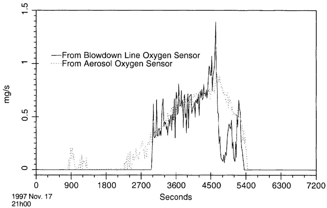
Figure 9: Hydrogen Production Rates Calculated from Oxygen Sensor Data
