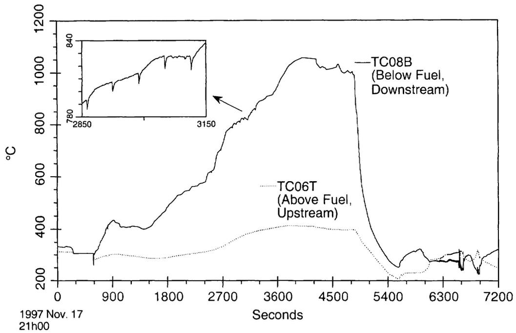
Figure 5: *Coolant Temperatures Above and Below Fuel*
