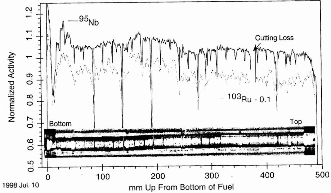
Figure 19:  $^{95}\text{Nb}$ ,  $^{103}\text{Ru}$  Activity Along Fuel Element
