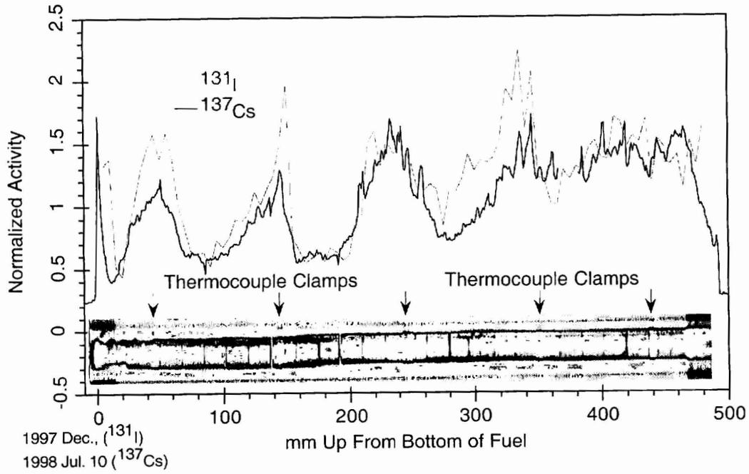
Figure 20:  $^{131}\text{I}$ ,  $^{137}\text{Cs}$  Activity Along Fuel Element
