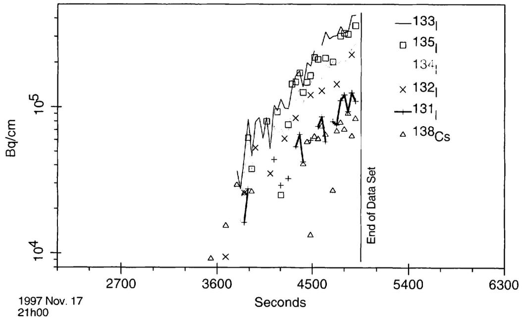
Figure 14: Iodine and Cesium in Liquid Side-Stream from Blowdown Tank
