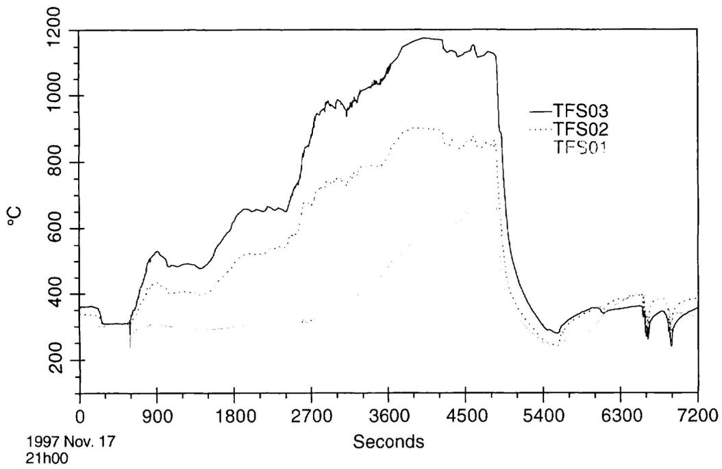
Figure 7: *Fuel-Sheath-Thermocouple Temperatures*
