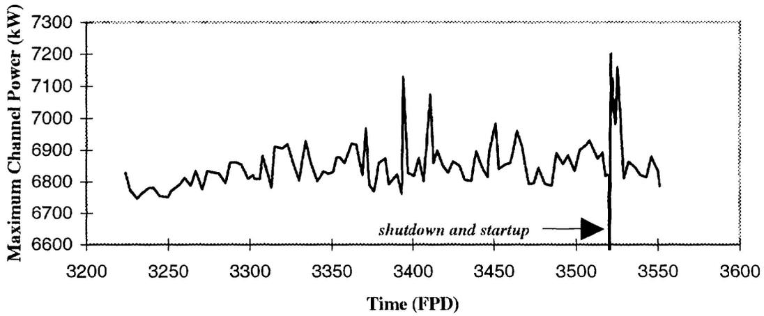
**Figure 3: Maximum Bundle Power (kW) vs. Time (FPD) for One-Year Core-Follow (including startup)**
