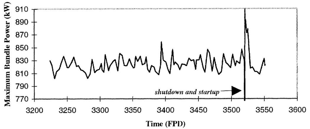
**Figure 4: Maximum Channel Power (kW) vs. Time (FPD) for Startup Period When Using Measured Poison Concentrations**
