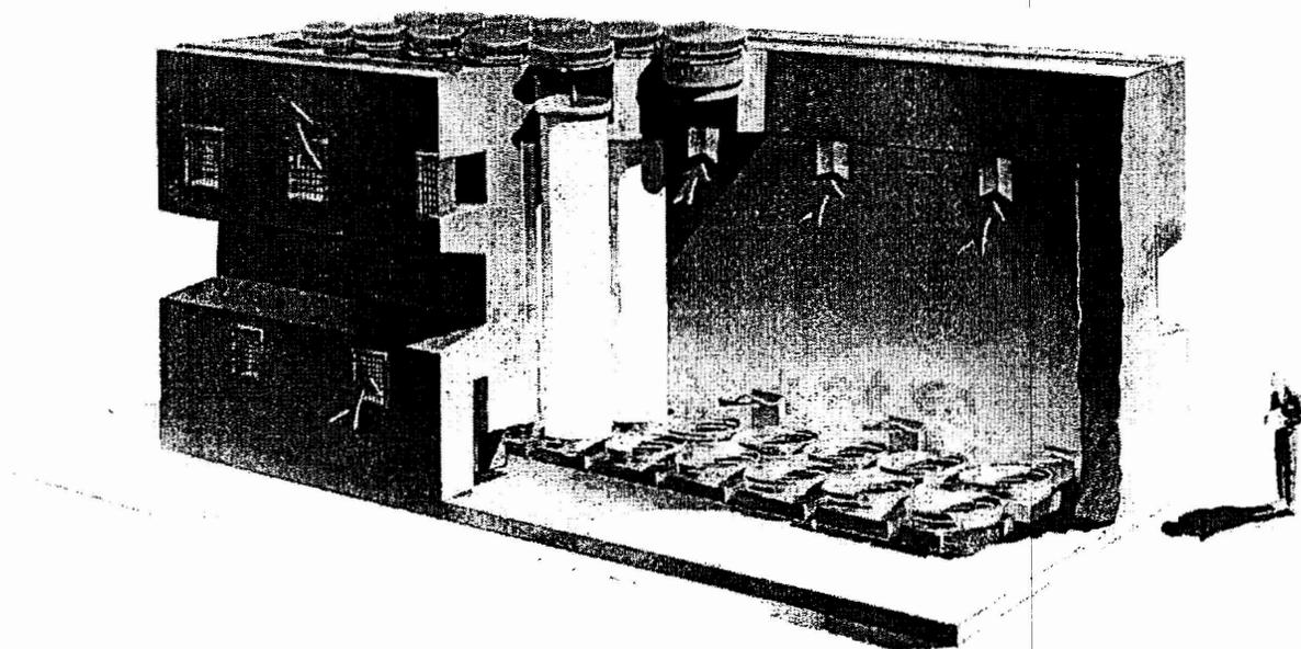
Figure 2. Diagram of air flow inside the CANSTOR module
