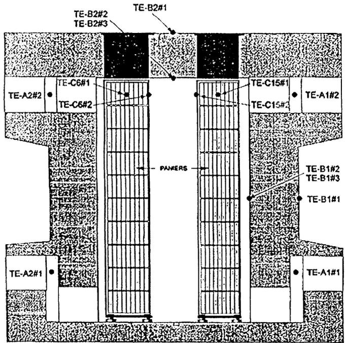
Figure 4. A cut of the Gentilly-2 CANSTOR module with two cylinders containing each 10 baskets
