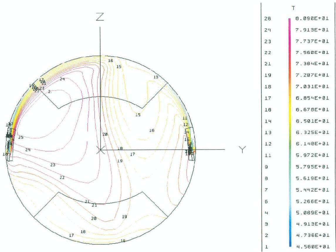
Figure 10b: Steady-State Temperature Contour for the Standard C6 Geometry in a Nozzle Plane (Reference Case).
