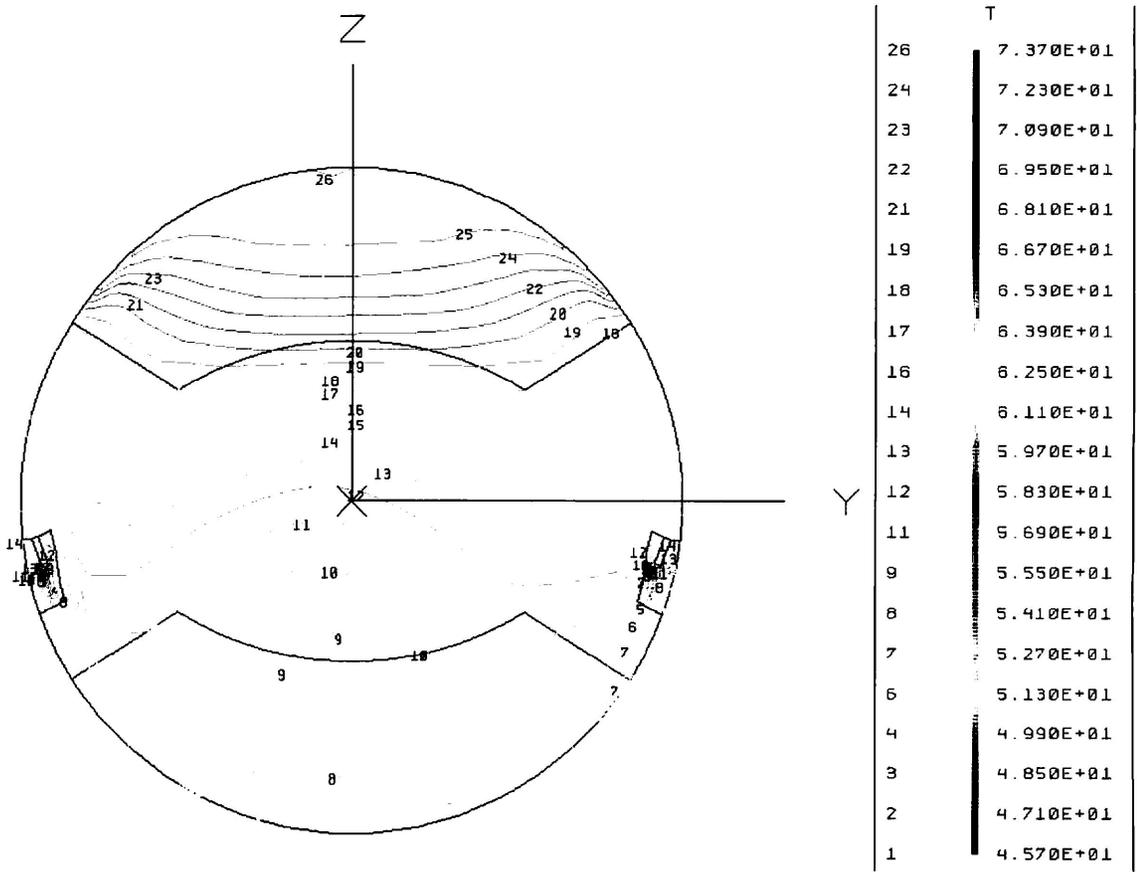
Figure 11b: Steady-State Temperature Contour for the Modified C6 Geometry at a Nozzle Plane (Reference Case).
