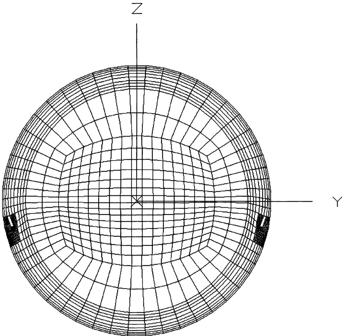
Figure 8: Modified CANDU 6 MODTURC\_CLAS Representation of the Moderator Cross Section (in the Y-Z Plane).
