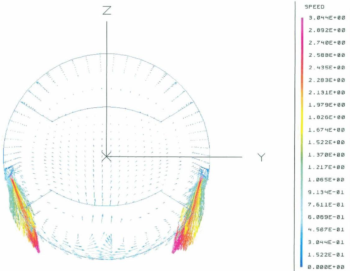
Figure 11a: Steady-State Velocity Vector Plot for the Modified C6 Geometry in a Nozzle Plane (Reference Case).
