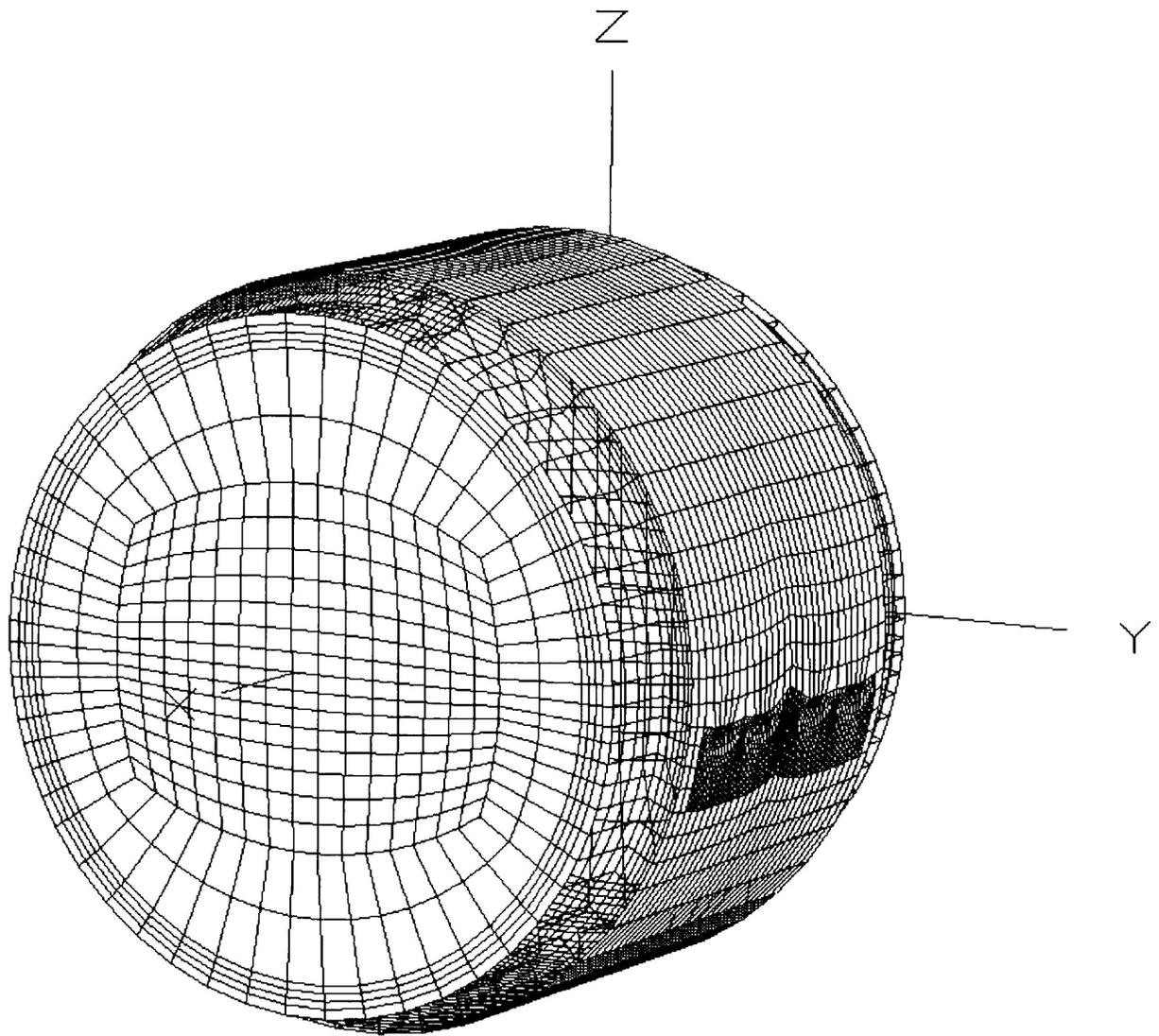
Figure 9: Three-Dimensional Wireframe Grid of the Modified CANDU 6 Geometry.
