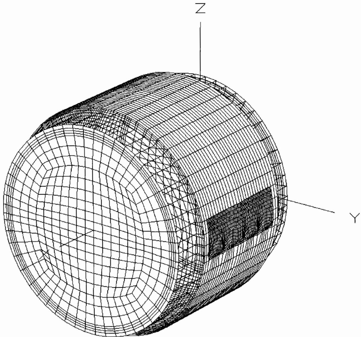
Figure 6: Three-Dimensional Wireframe Grid of the Standard CANDU 6 Geometry.
