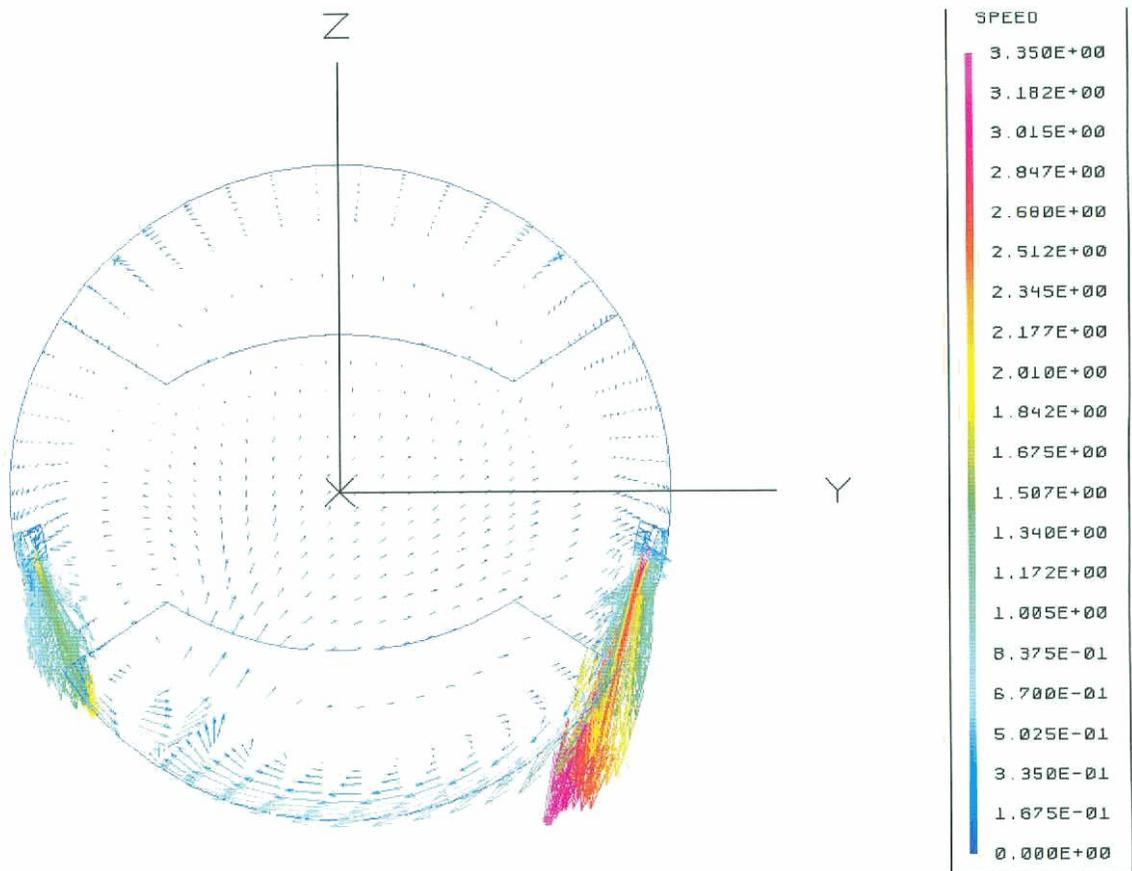
Figure 12a: Steady-State Velocity Vector Plot for the Modified C6 Design in a Nozzle Plane (Mass Flow Imbalance Case 2).
