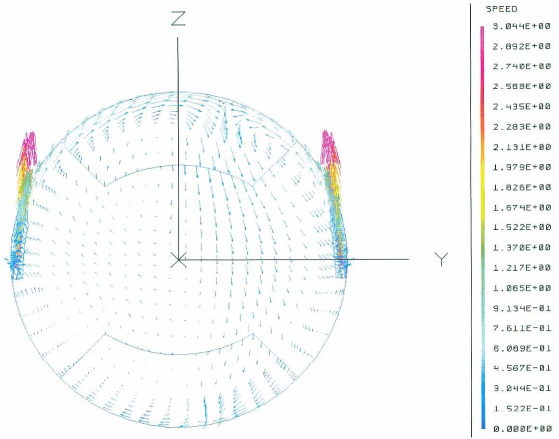
Figure 10a: Steady-State Velocity Vector Plot for the Standard C6 Geometry in a Nozzle Plane (Reference Case).
