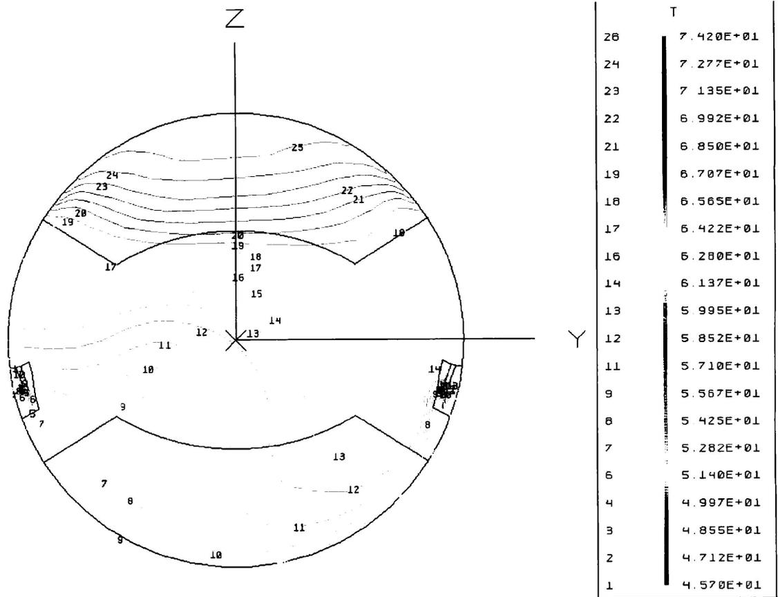
Figure 12b: Steady-State Temperature Contour for the Modified C6 Design in a Nozzle Plane (Mass Flow Imbalance Case 2).
