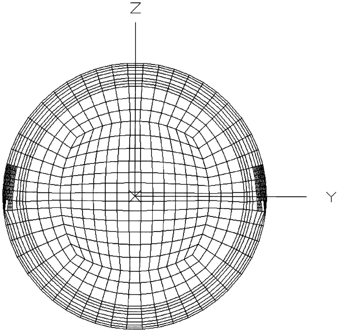
Figure 5: Standard CANDU 6 MODTURC\_CLAS Representation of the Moderator Cross Section (in the Y-Z Plane).
