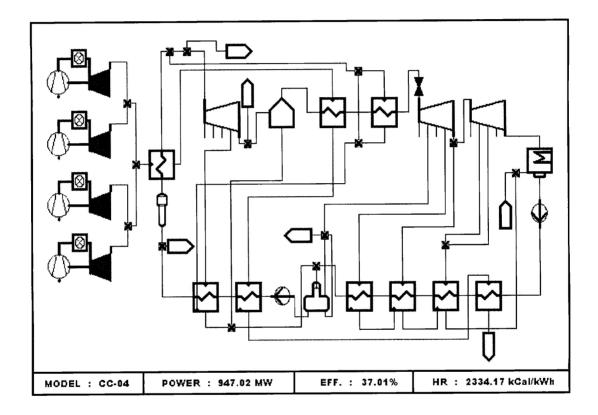
Figure 7 GateCycle Model of CANDU Gas-Turbine Combined Cycle (Case 6)
