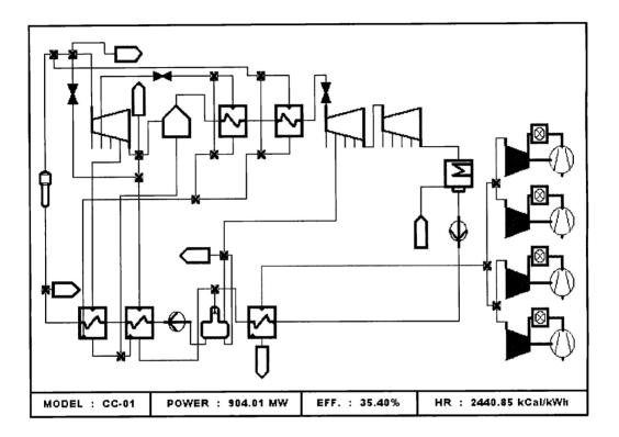
Figure 4 GateCycle Model of CANDU Gas-Turbine Combined Cycle (Case 3)
