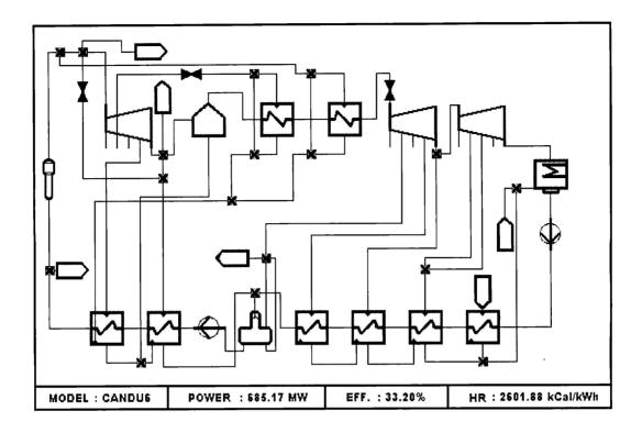
Figure 2 GateCycle Model of Conventional CANDU 6 BOP (Case 1)
