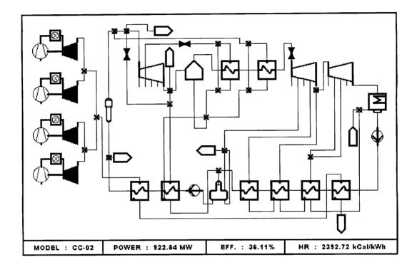
Figure 5 GateCycle Model of CANDU Gas-Turbine Combined Cycle (Case 4)
