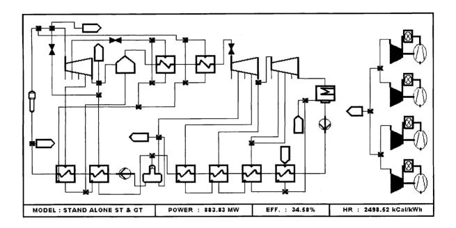
Figure 3 GateCycle Model of Conventional CANDU 6 BOP and Stand-Alone Gas-Turbine Engines (Case 2)
