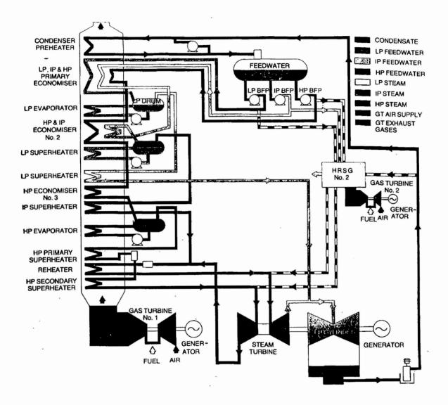
Figure 1 Schematic Diagram of a 690 MW Combined-Cycle Power Station
