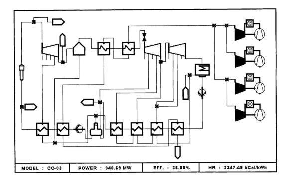
Figure 6 GateCycle Model of CANDU Gas-Turbine Combined Cycle (Case 5)
