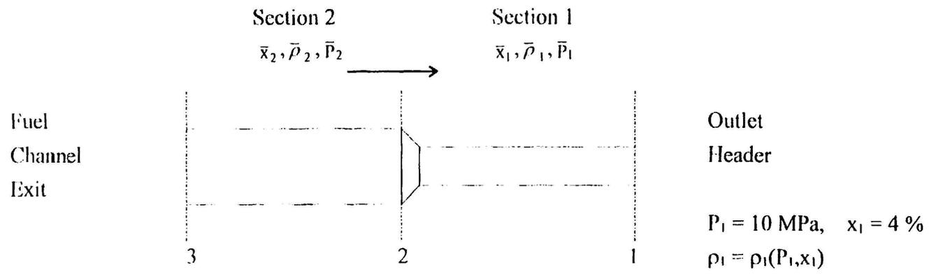
FIG. 4 CONFIGURATION OF OUTLET FEEDER
