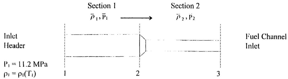
FIG. 3 CONFIGURATION OF INLET FEEDER
