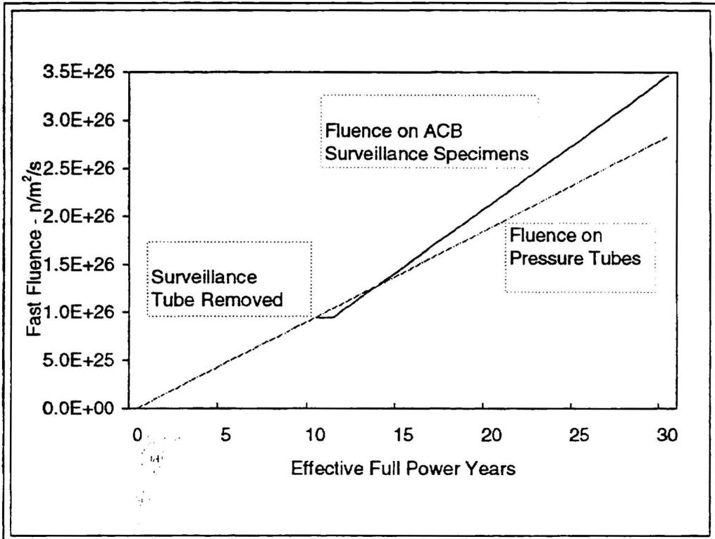
FIGURE 8: TYPICAL FLUENCE ACCUMULATION:
