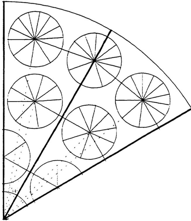
**Figure 2: Sample Geometrical Representation used in FACTAR 2.0 (LOCA) for a 37-element Bundle (two 1/12<sup>th</sup> symmetric wedges)**
