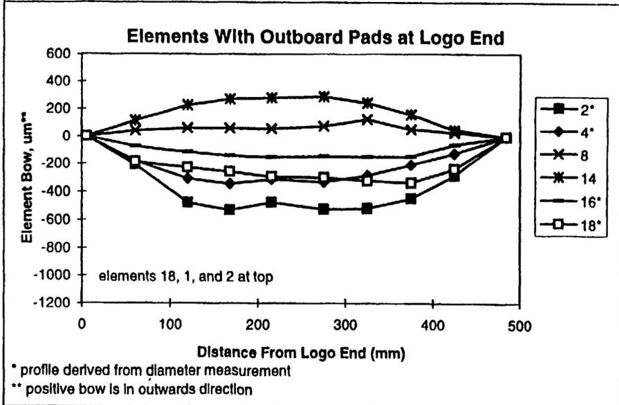
**FIGURE 6: Element Bow of SECTIONED IRRADIATED Bundle From BNGS-8 S22 (Manufacturer B - J81764C)**
