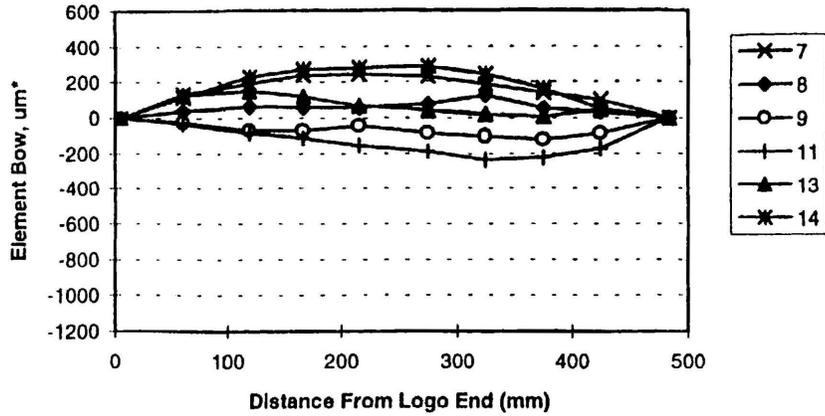
**Bow Measured From Element in 12 O'clock Position
