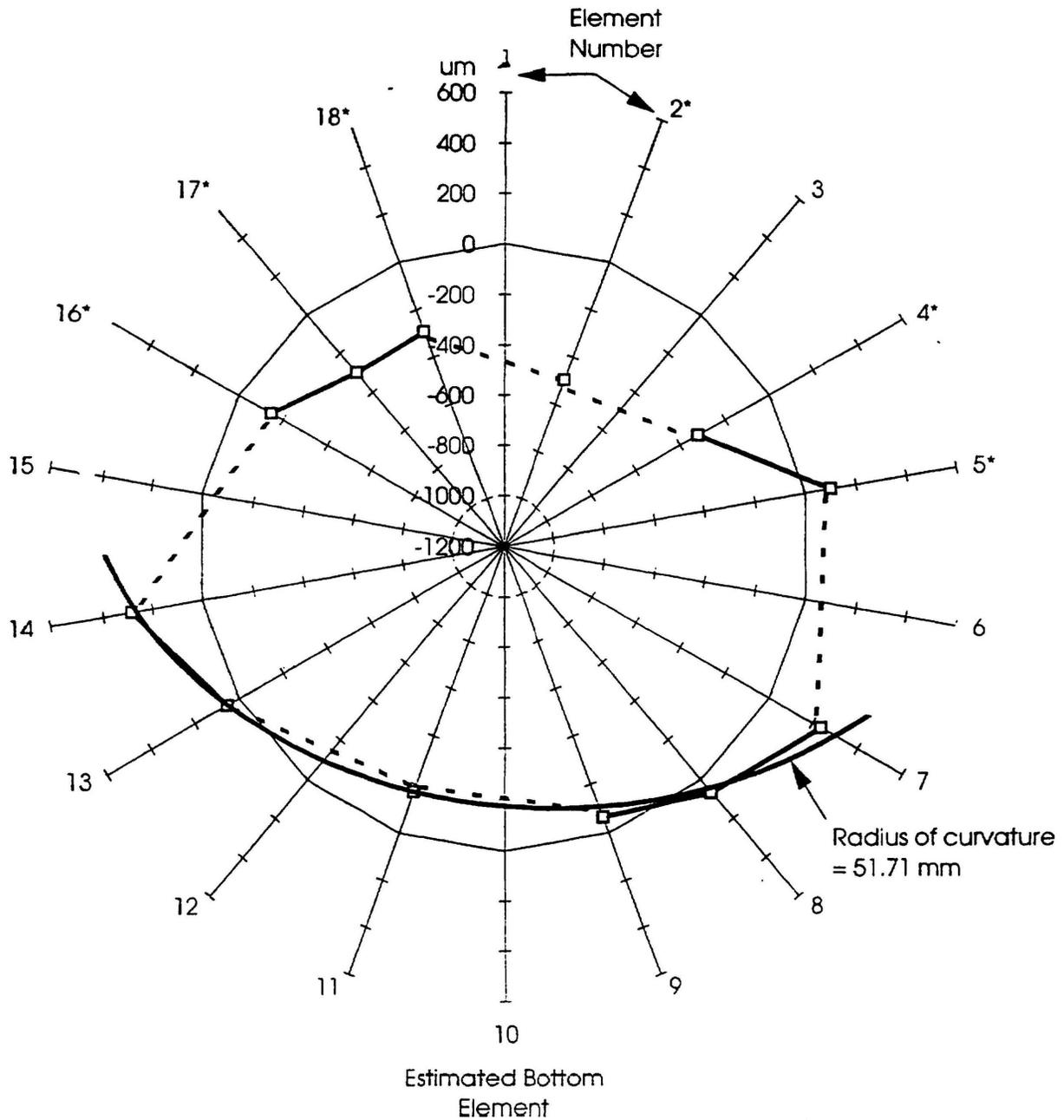
\* Profiles derived from diameter measurements
