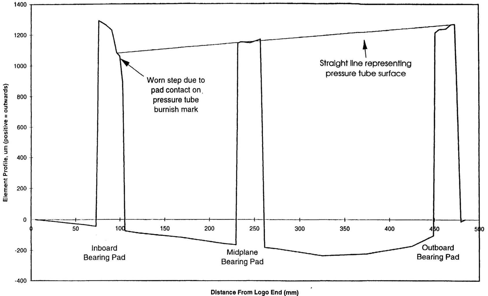
**FIGURE 8: Linearity of Worn Bearing Pad Surfaces Measured From Intact Irradlated Bundle**
