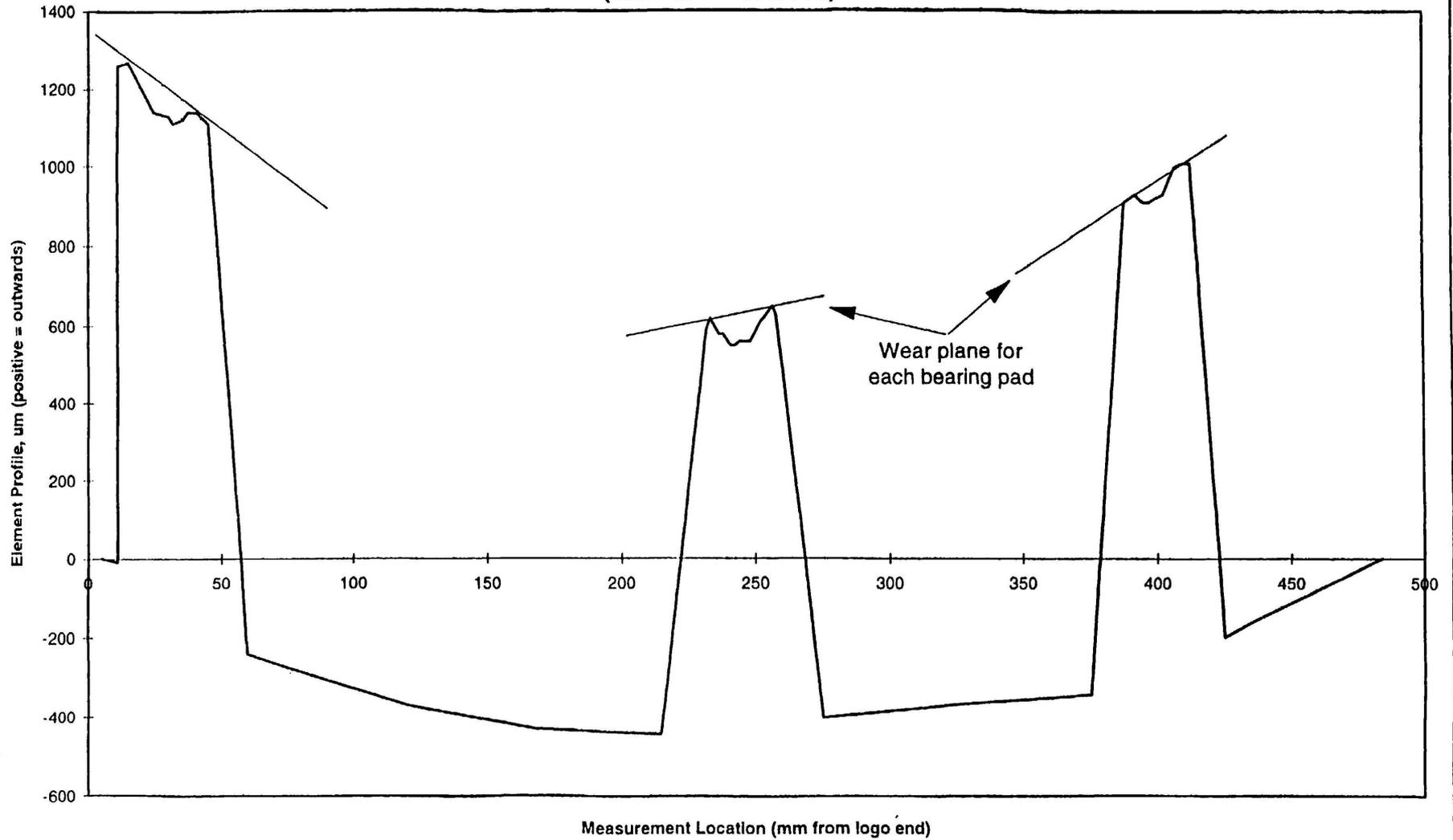
FIGURE 1: Inward Bow and Non-Linearity of Bearing Pad Wear Measured From Separated Irradiated Element
