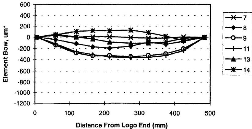
**FIGURE 10: Effect of Sag Caused by Gravity on Element Profiles From Intact Irradiated Bundle**
