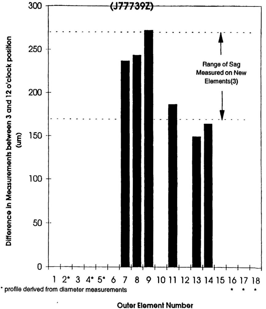
**FIGURE 11: Effect of Gravity on Element Sag**
