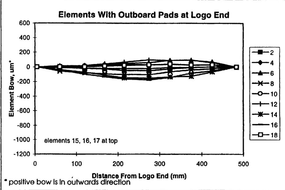
**FIGURE 4: Outer Element Profiles From Manufacturer A Bundle After DNGS-3 ZPH test(3) (K42148Z)**
