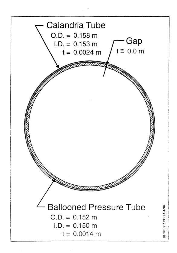
FIGURE 2 TEST ELEMENT CROSS SECTION
