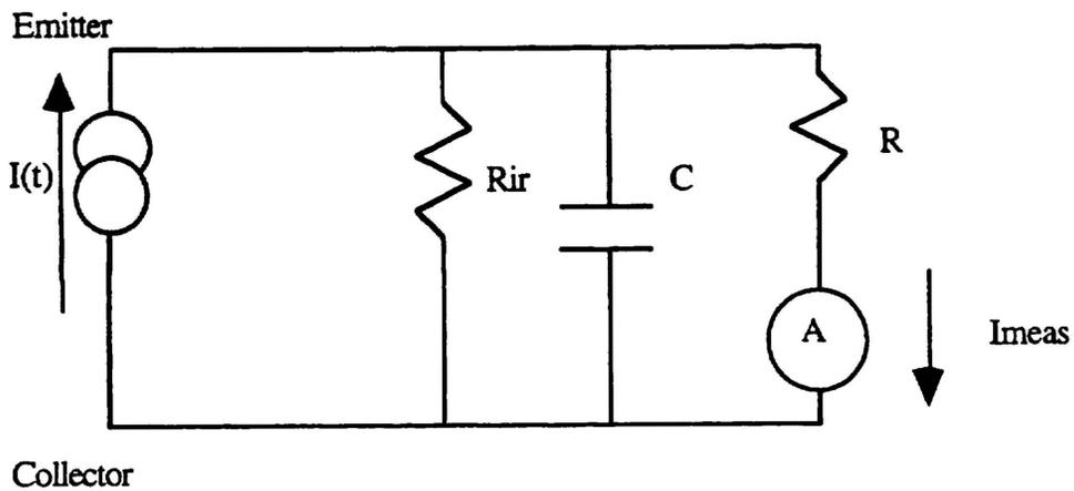
FIGURE 3. ELECTRICAL MODEL OF AN IN-CORE FLUX DETECTOR
