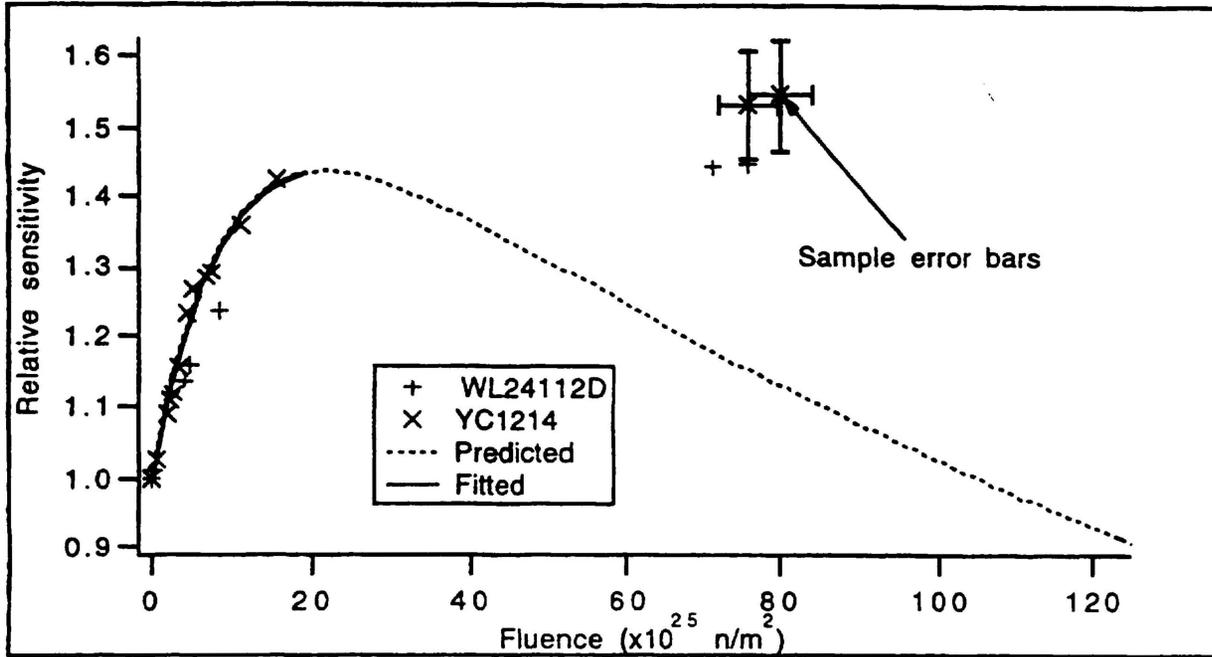
FIGURE 5. INCONEL SIR MEASURED AND PREDICTED CHANGE IN SENSITIVITY WITH FLUENCE
