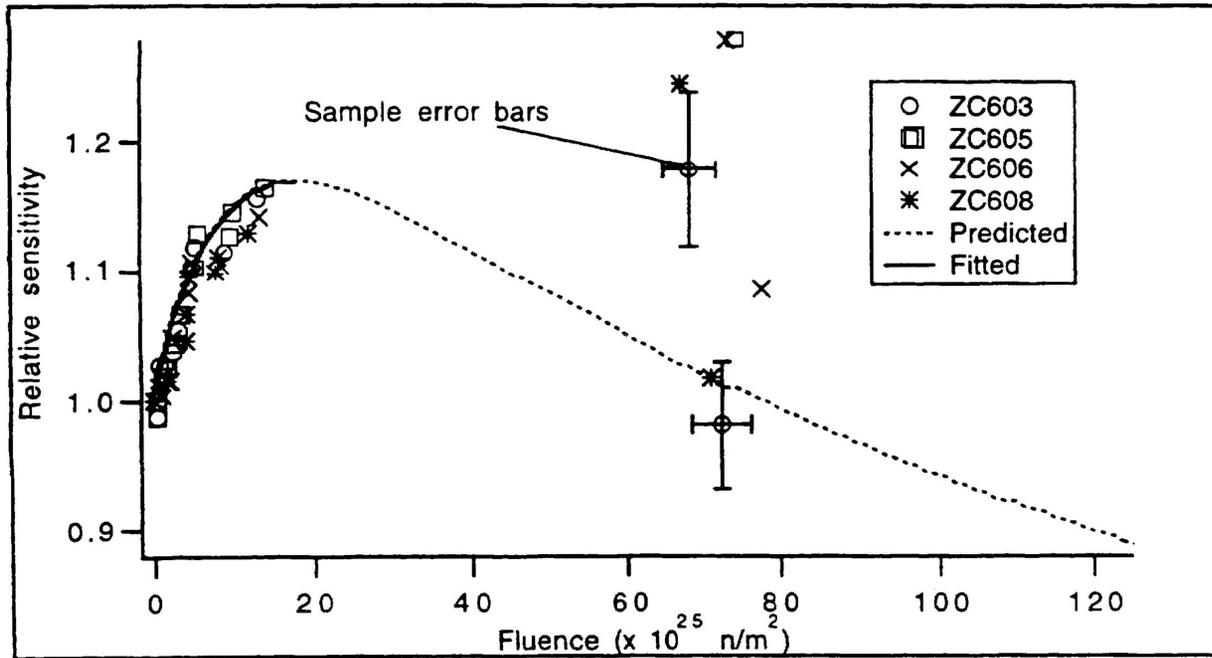
FIGURE 6. PLATINUM-CLAD INCONEL SIR MEASURED AND PREDICTED CHANGE IN SENSITIVITY WITH FLUENCE
