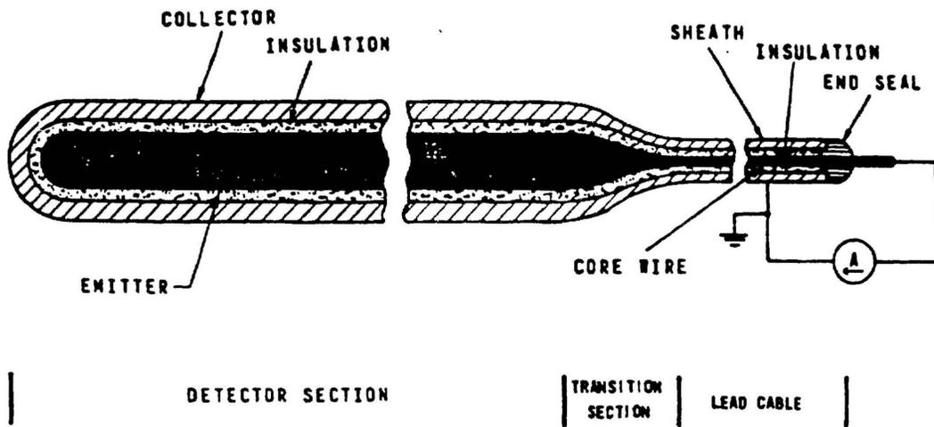
FIGURE 1. IN-CORE FLUX DETECTOR CONSTRUCTION
