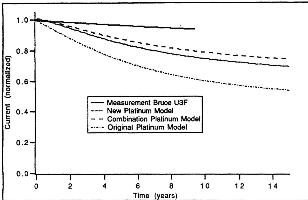
FIGURE 7 PLATINUM MEASURED, PREDICTED, AND MODIFIED CHANGE IN SENSITIVITY WITH FLUENCE
