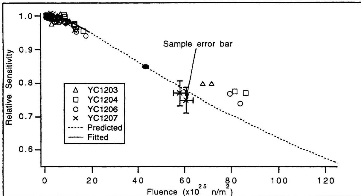
FIGURE 4. VANADIUM SIR MEASURED AND PREDICTED CHANGE IN SENSITIVITY WITH FLUENCE
