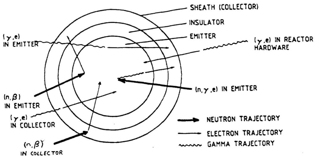
FIGURE 2. ATOMIC INTERACTIONS IN AN IN-CORE FLUX DETECTOR
