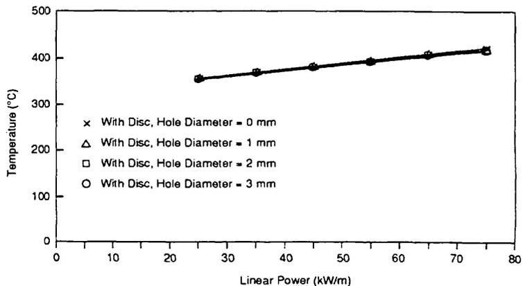
Figure 12 Sheath Temperature at Disc Interface,  $T_{sd}$
