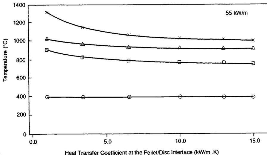
Figure 5 Fuel Temperatures vs Pellet/Disc Heat Transfer
