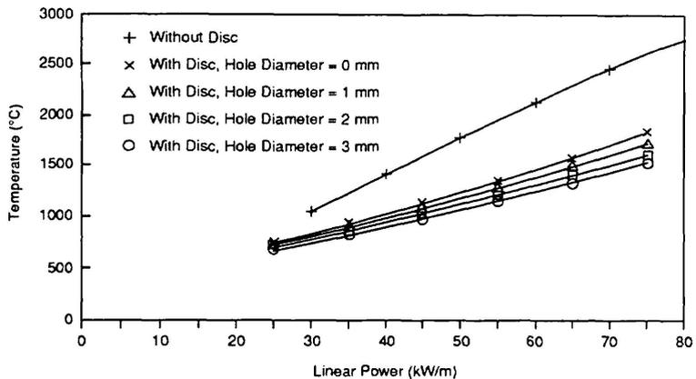
Figure 11 Maximum Temperature in the Pellet at the Pellet/Disc Interface,  $T_{pd}$
