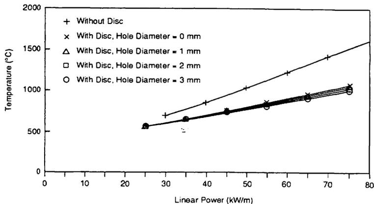
Figure 10 Cross-Section Average Temperature at the End Plane of the Pellet,  $T_{cs}$
