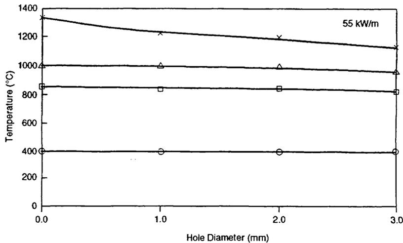
Figure 8 Fuel Temperatures vs Central Hole Diameter
