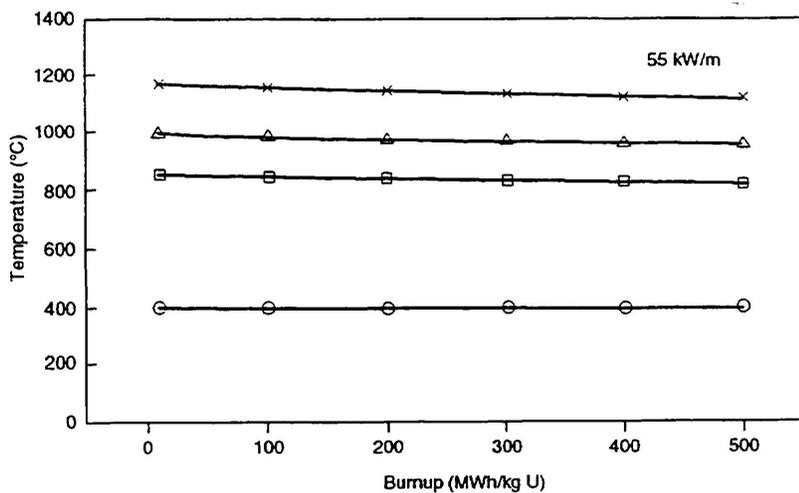
Figure 4 Fuel Temperatures vs Element Burnup
