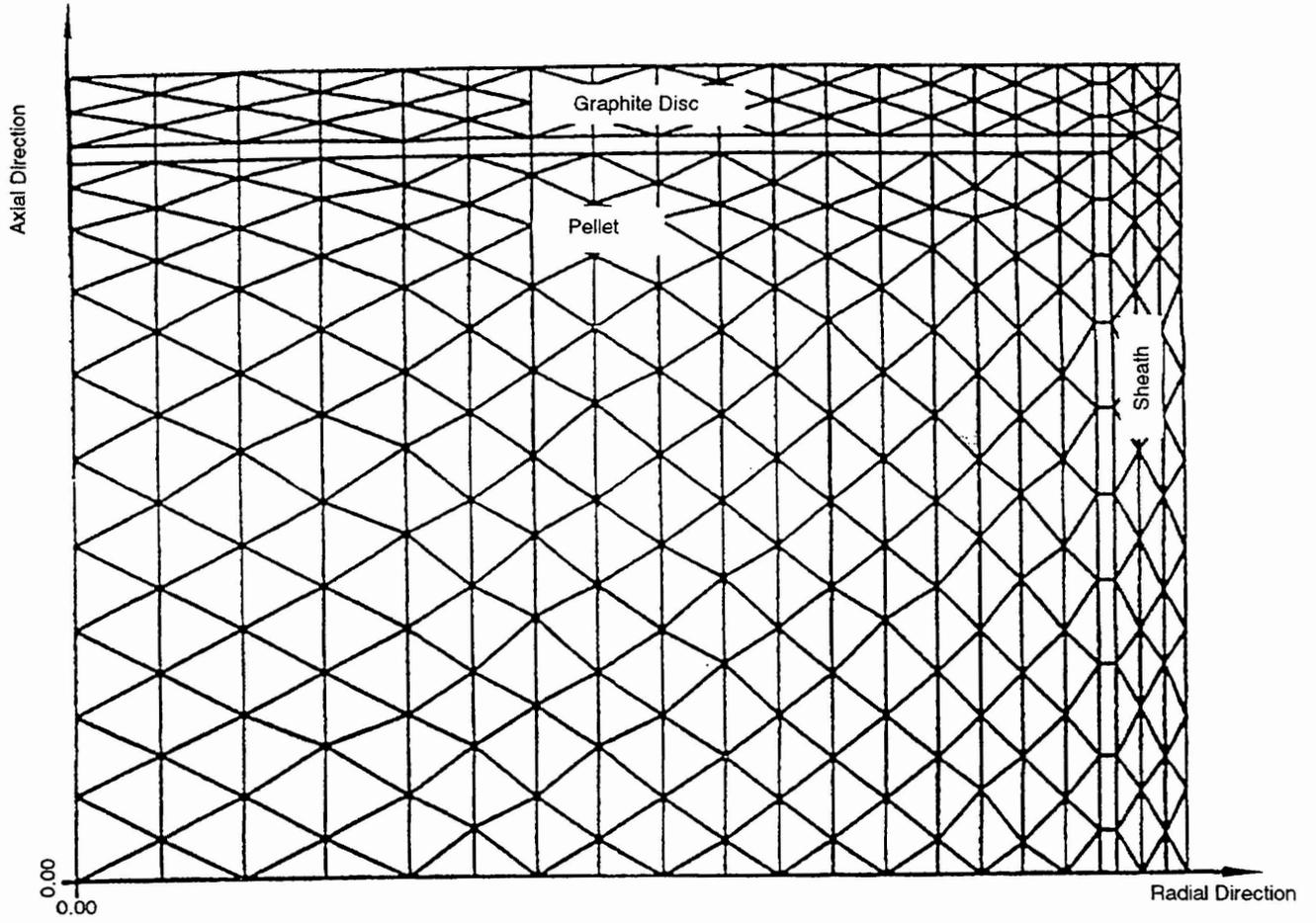
Figure 2 Finite Element Mesh of the Model
