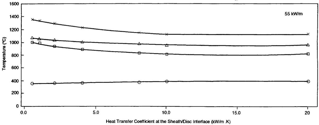
Figure 7 Fuel Temperatures vs Sheath/Disc Heat Transfer
