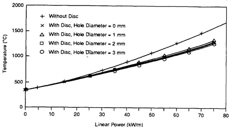
Figure 9 Volume-Average Temperature in the Pellet,  $T_v$
