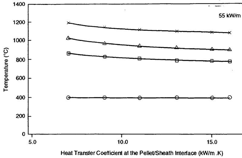
Figure 6 Fuel Temperatures vs Pellet/Sheath Heat Transfer
