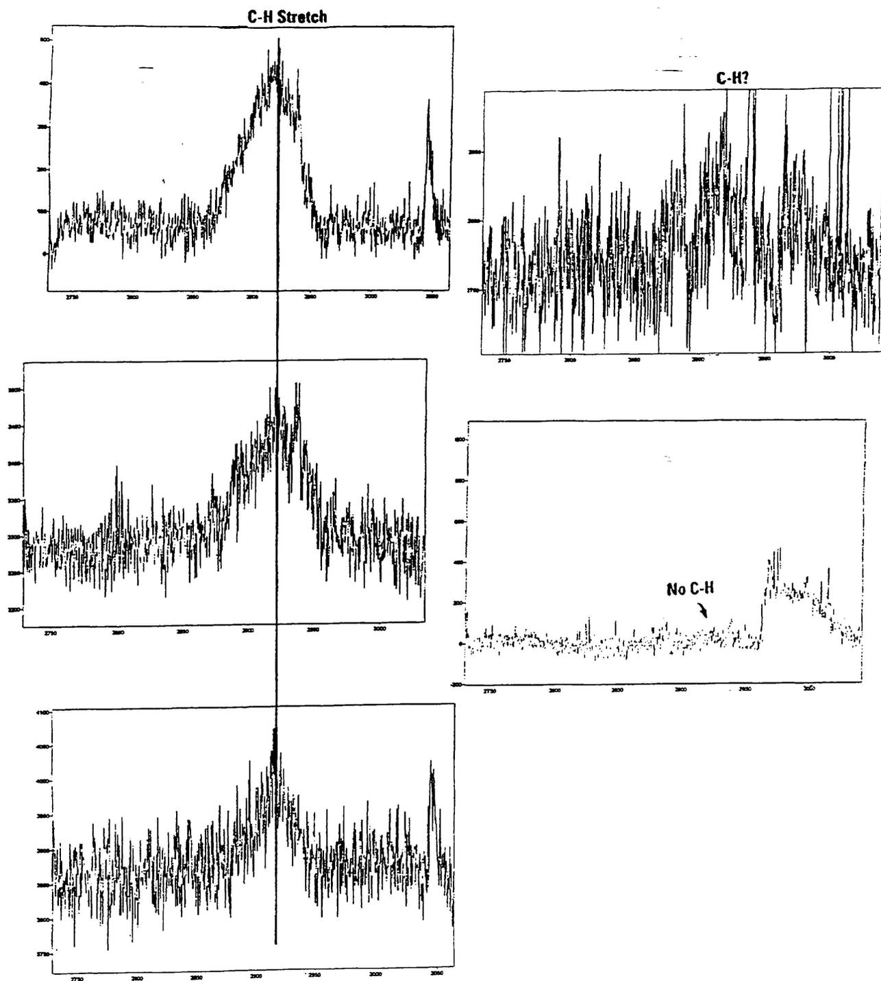
FIGURE 5: RAMAN SPECTRA OBTAINED FROM CANLUB (DAG-154 COATING) BAKED AT TEMPERATURES RANGING FROM 320 TO 440°C. THE TWO ON THE RIGHT HAND SIDE WERE AT THE HIGHEST TEMPERATURES.
