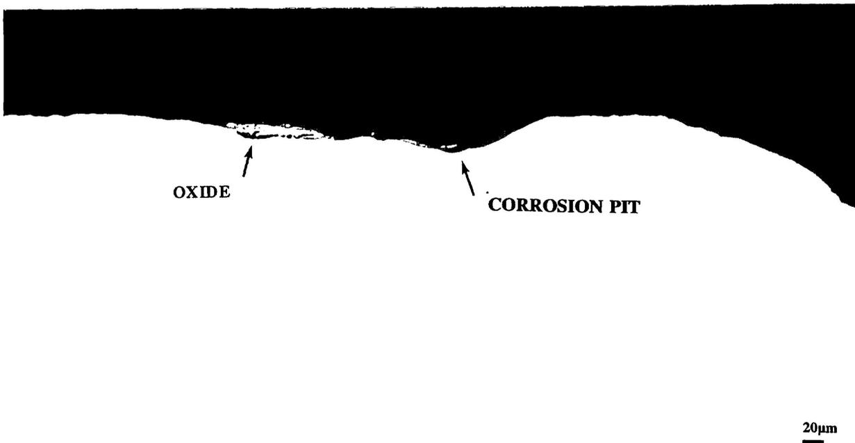
FIGURE 6: THE LARGEST CORROSION PIT OBSERVED (~0.5 mm IN DIAMETER x 38 μm DEEP) ON THE CONTACT SURFACE OF A T-PAD. NOTE THE PATCH OF OXIDE IN THE PIT REGION (200X).
