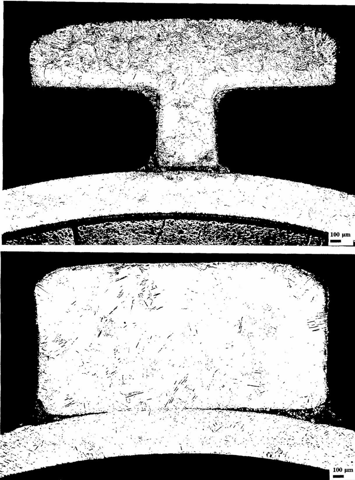
FIGURE 4: COMPARISON OF A T-PAD AND A STANDARD BEARING PAD, ETCHED TO REVEAL HYDRIDE/DEUTERIDE DISTRIBUTION (50X).
