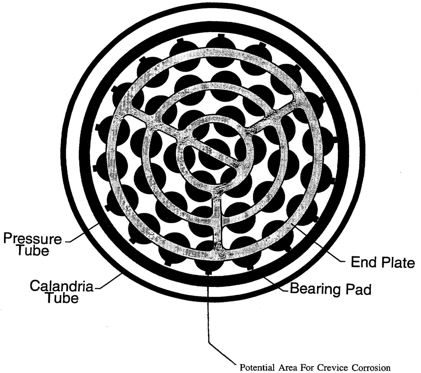
FIGURE 1: CROSS-SECTION OF BUNDLE, PRESSURE TUBE & CALANDRIA TUBE
