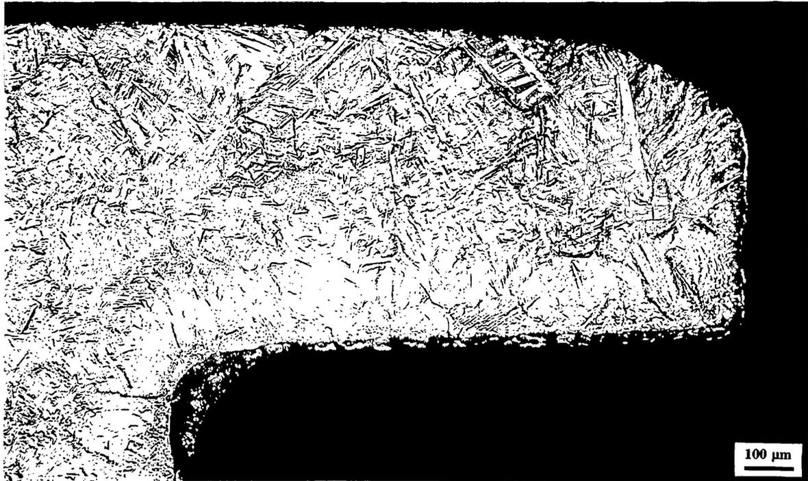
FIGURE 5: THE T-PAD DISPLAYING THE GREATEST AMOUNT OF HYDRIDE/DEUTERIDE OBSERVED (100X).
