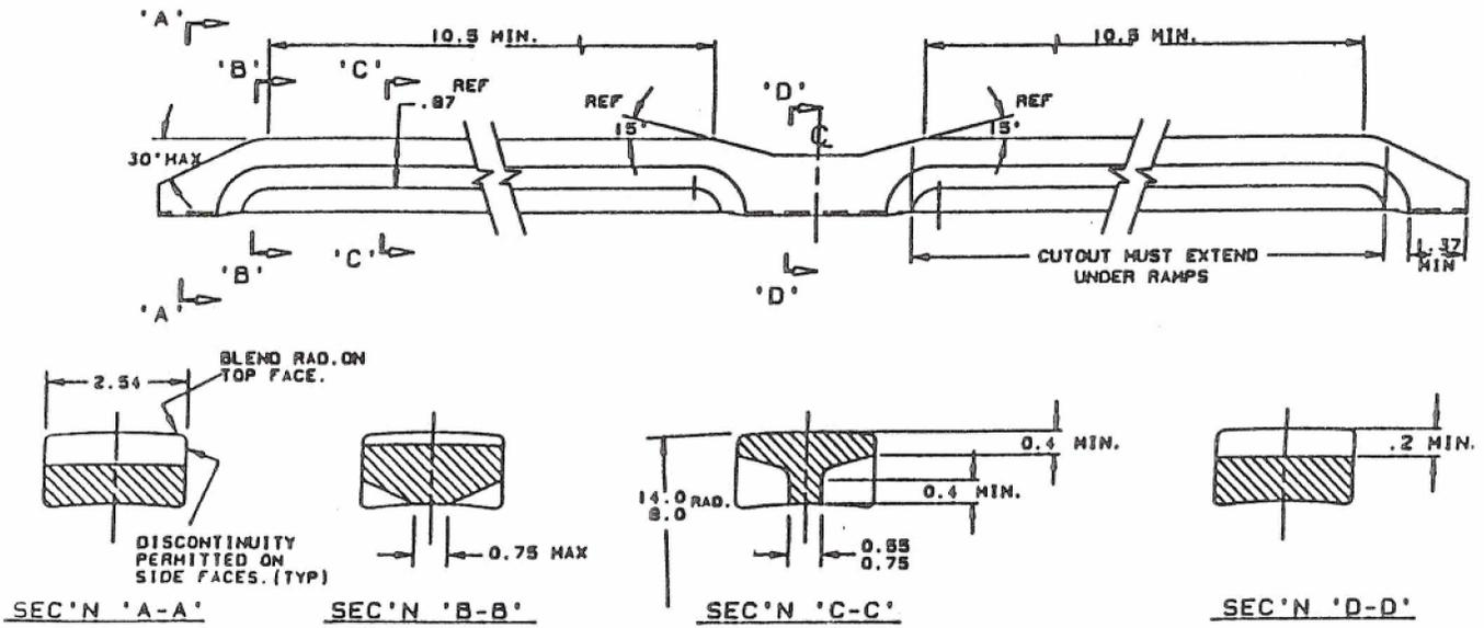
FIGURE 2: T-PAD BEARING PAD DESIGN
