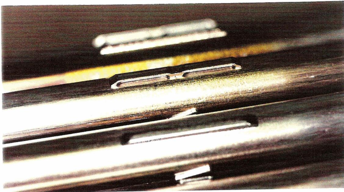
FIGURE 3: T-PAD BEARING PADS AS INSTALLED ON A CANDU BUNDLE
