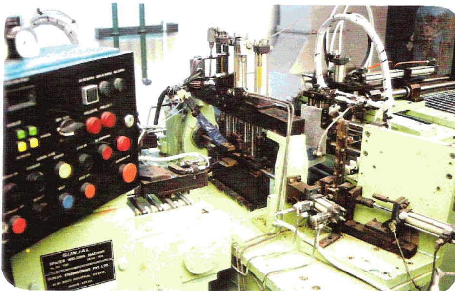
FIG-3 CLOSE-UP OF SPACER PAD WELDING MACHINE
