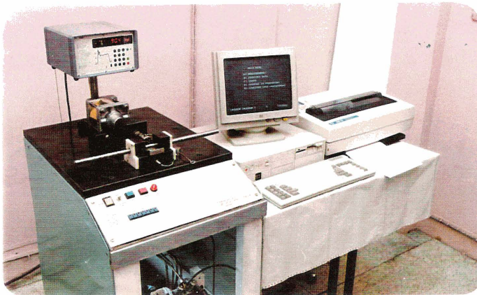
FIG.-8. SHEAR STRENGTH TESTING MACHINE
