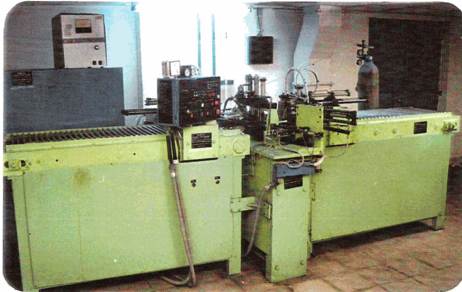
FIG-2 AUTOMATIC SPACER PAD WELDING MACHINE
