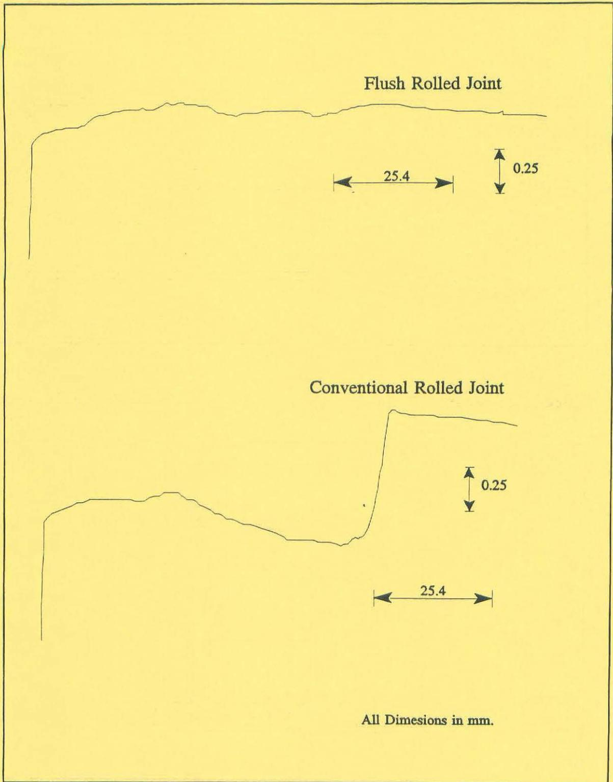
Figure 5: Axial Profiles of the Rolled Joint Regions
