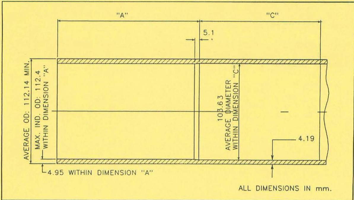
Figure 2: Pressure Tube Geometry - Spools for LCRJ Fabrication
