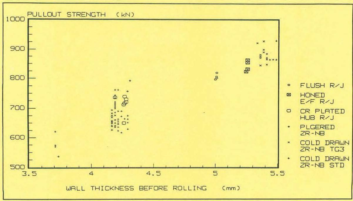
Figure 6: Hot Pressurized Pullout Test Results
