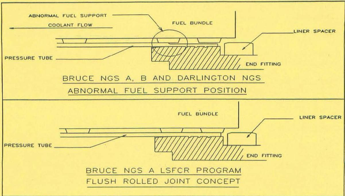
Figure 1: Abnormal Fuel Support and Flush Rolled Joint Concept
