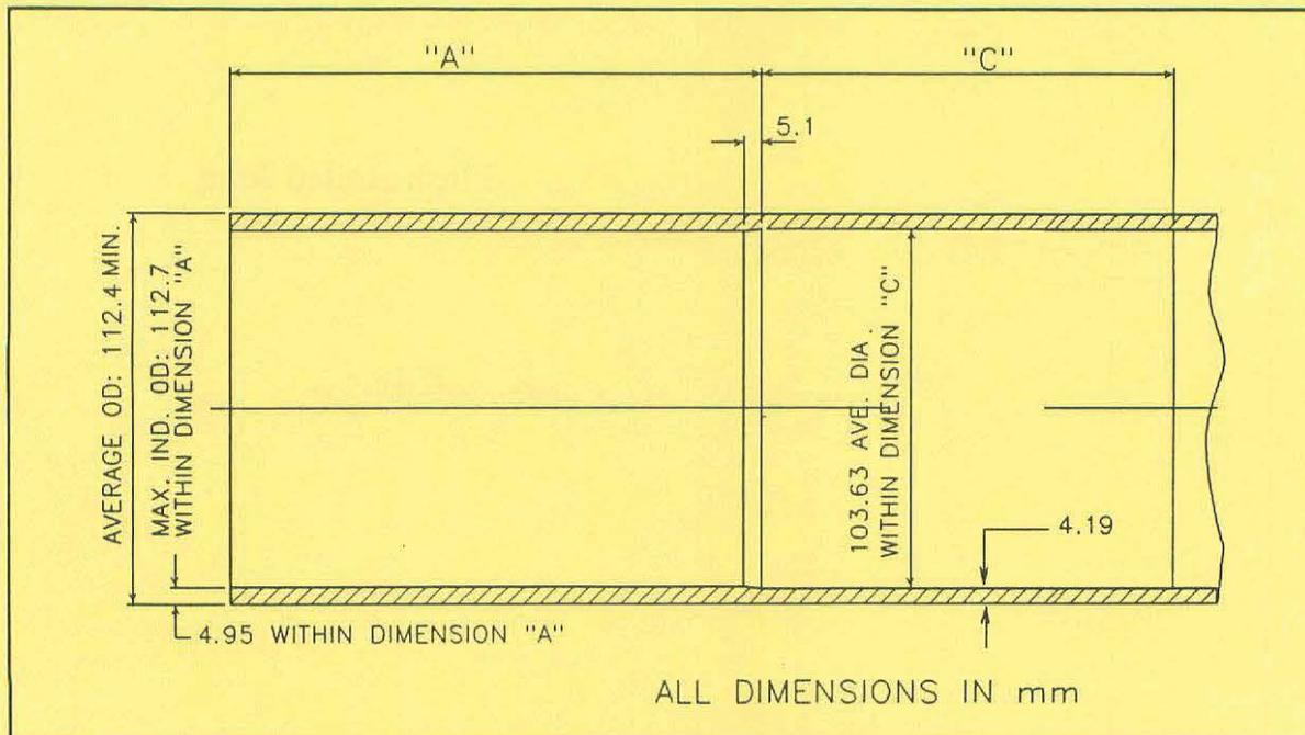
Figure 3: Pressure Tube Geometry - Spools for ZCRJ Fabrication
