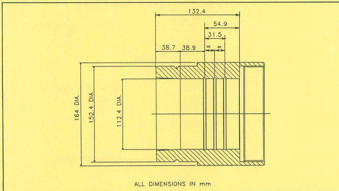
Figure 4: End Fitting Hub Geometry
