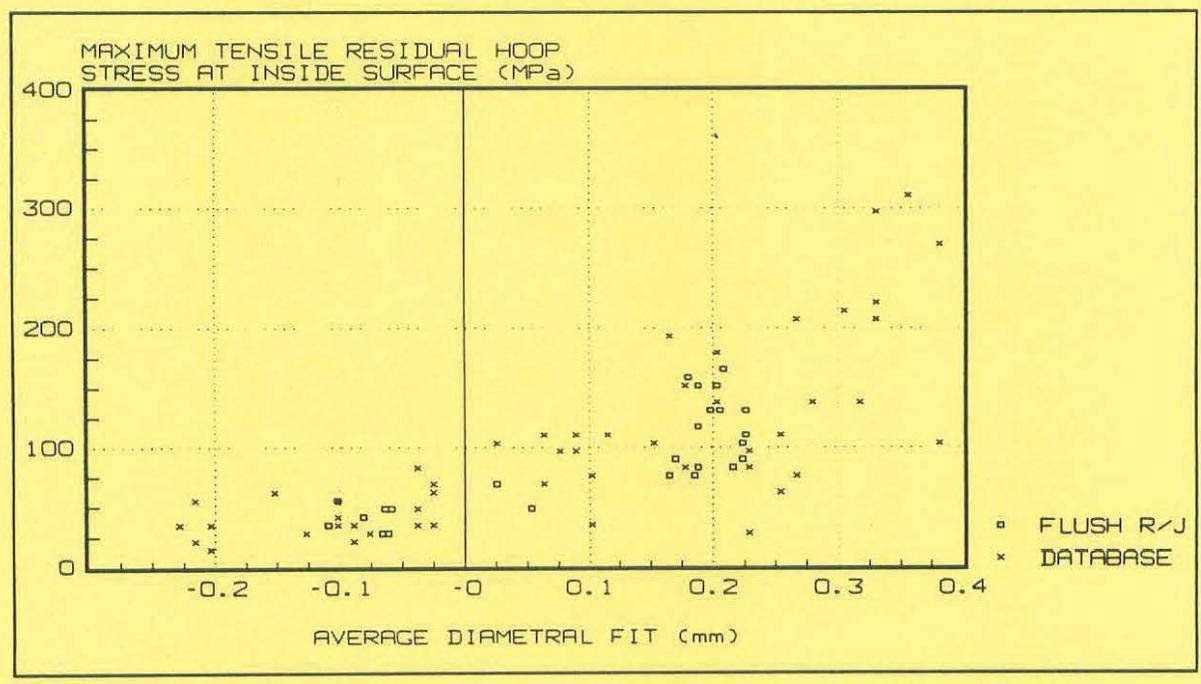
Figure 7: Maximum Tensile Residual Hoop Stress at the Inside Surface of the Pressure Tube
