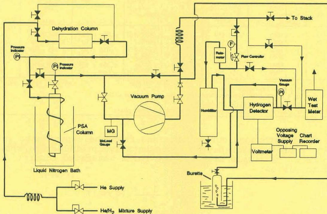
Figure 1: Schematic of the PSA Experimental Apparatus
