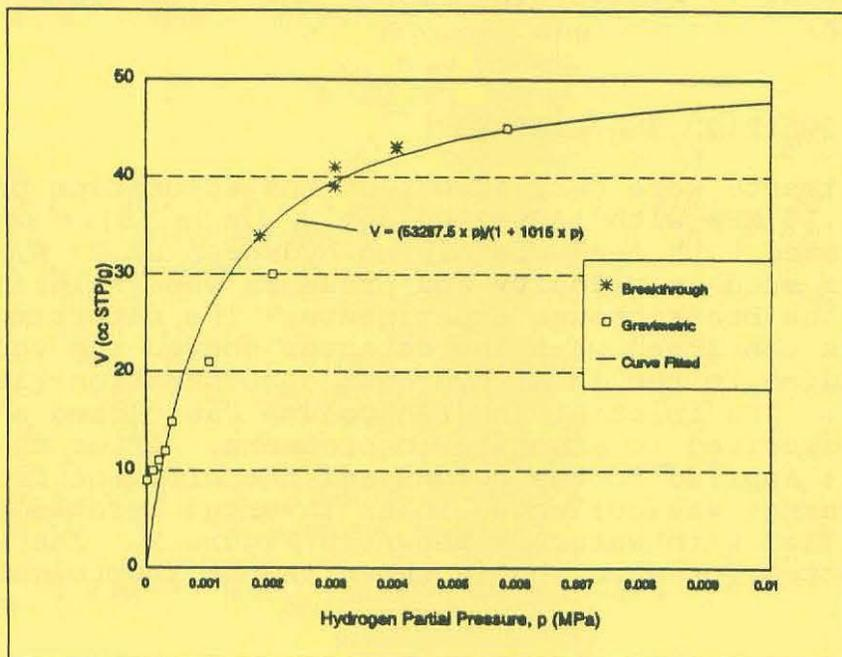
Figure 3: Comparison of Breakthrough and Gravimetric Equilibrium Data of Hydrogen on Molecular Sieve 5A at 77K
