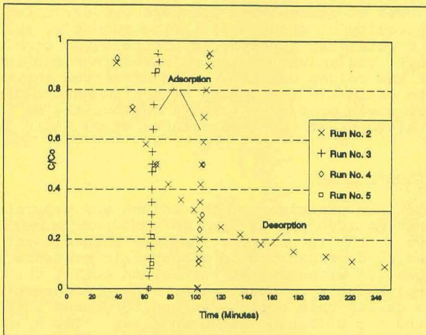
Figure 2: Reproducibility of the Experimental Adsorption and Desorption Breakthrough Curves
