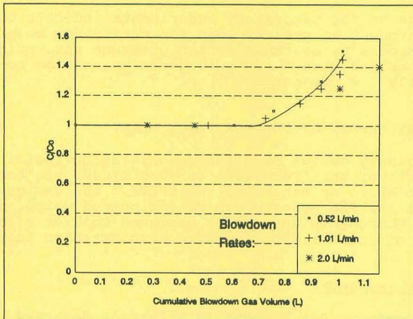
Figure 5: Volume and Composition of Effluent Gas During Blowdown of An Equilibrated Bed
