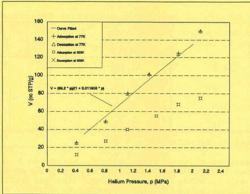
Figure 4: Helium Isotherms on Molecular Sieve 5A at 77 K and 303 K
