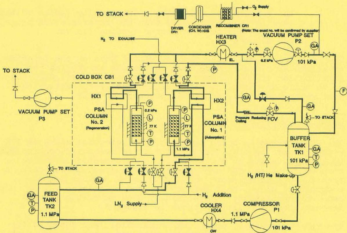
Figure 6: Preliminary Schematic for PSA Demonstration Facility
