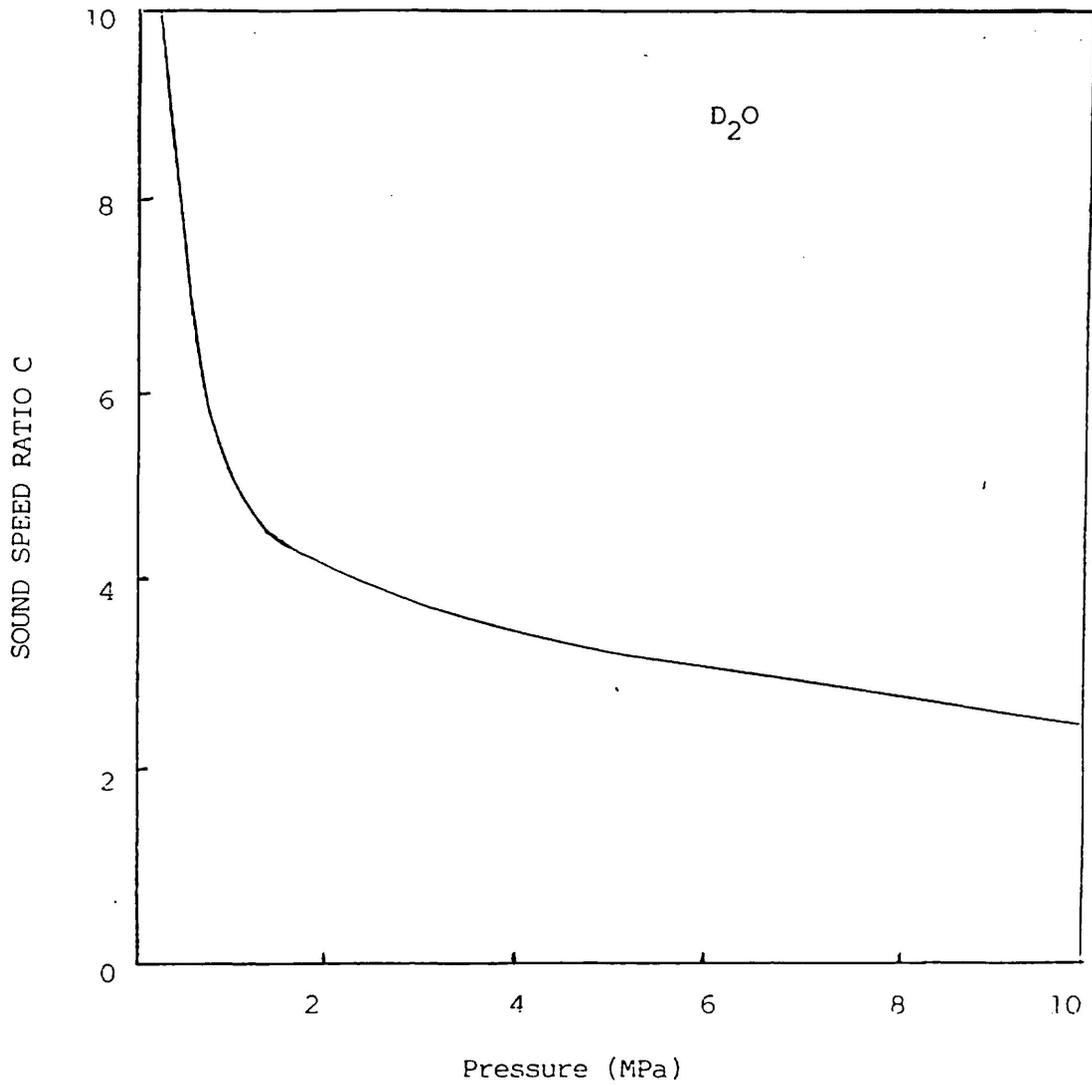
Figure 5. Ratio of the homogeneous frozen and homogeneous equilibrium sound speeds for heavy water at low void fraction
