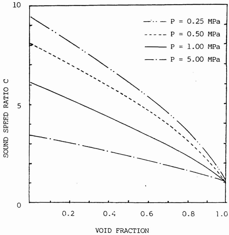
Figure 6. Ratio of the homogeneous frozen and homogeneous equilibrium sound speeds as a function of pressure
