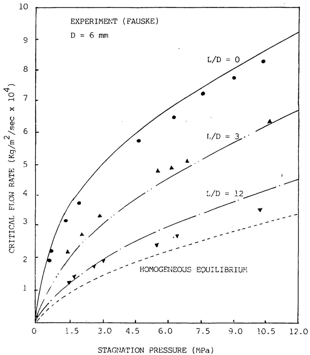
Figure 10. Critical flow rates as a function of L/D
