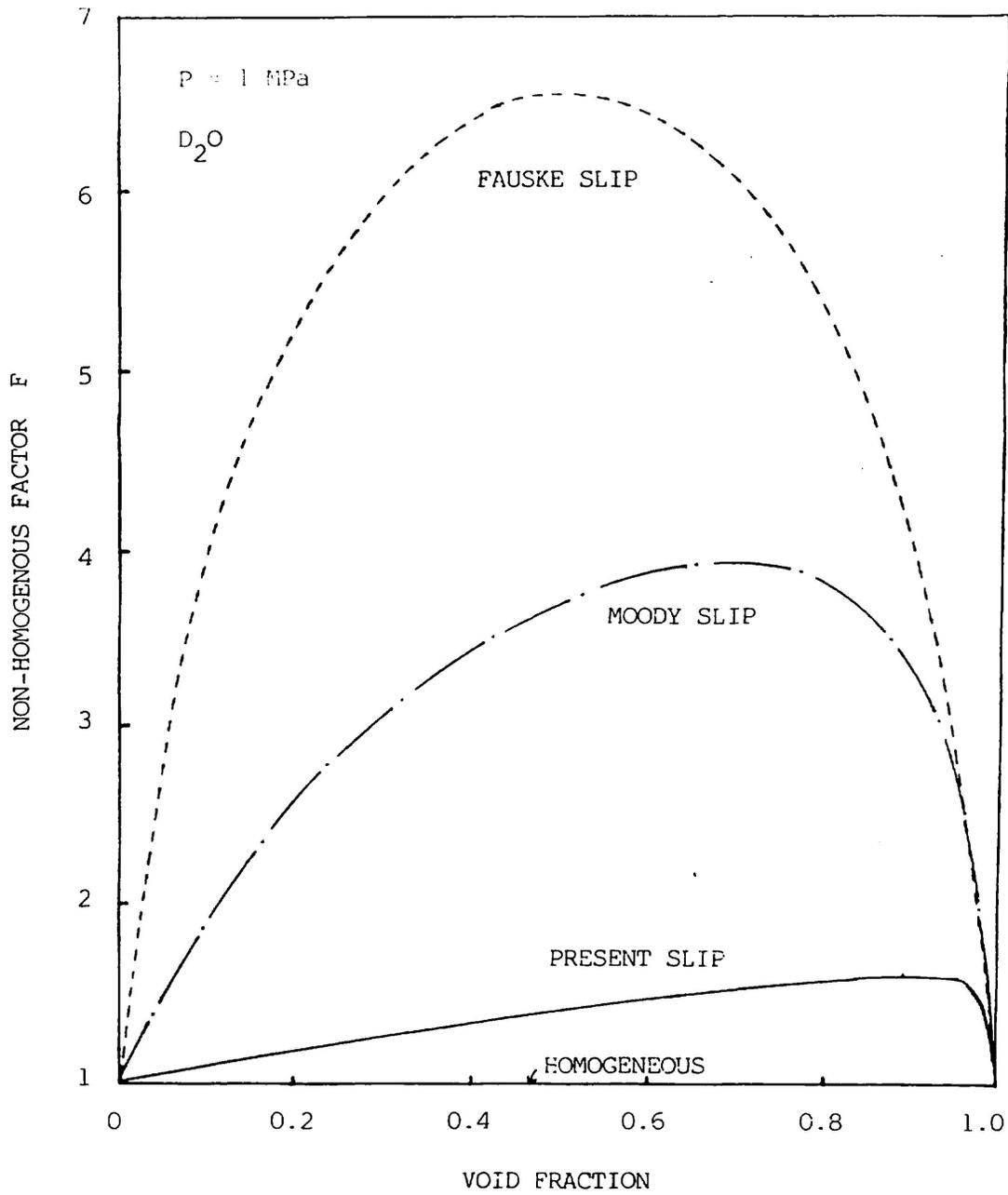
Figure 2. The non-homogeneous factor  $F$  as a function of void fraction at  $P = 1 \text{ MPa}$  of heavy water
