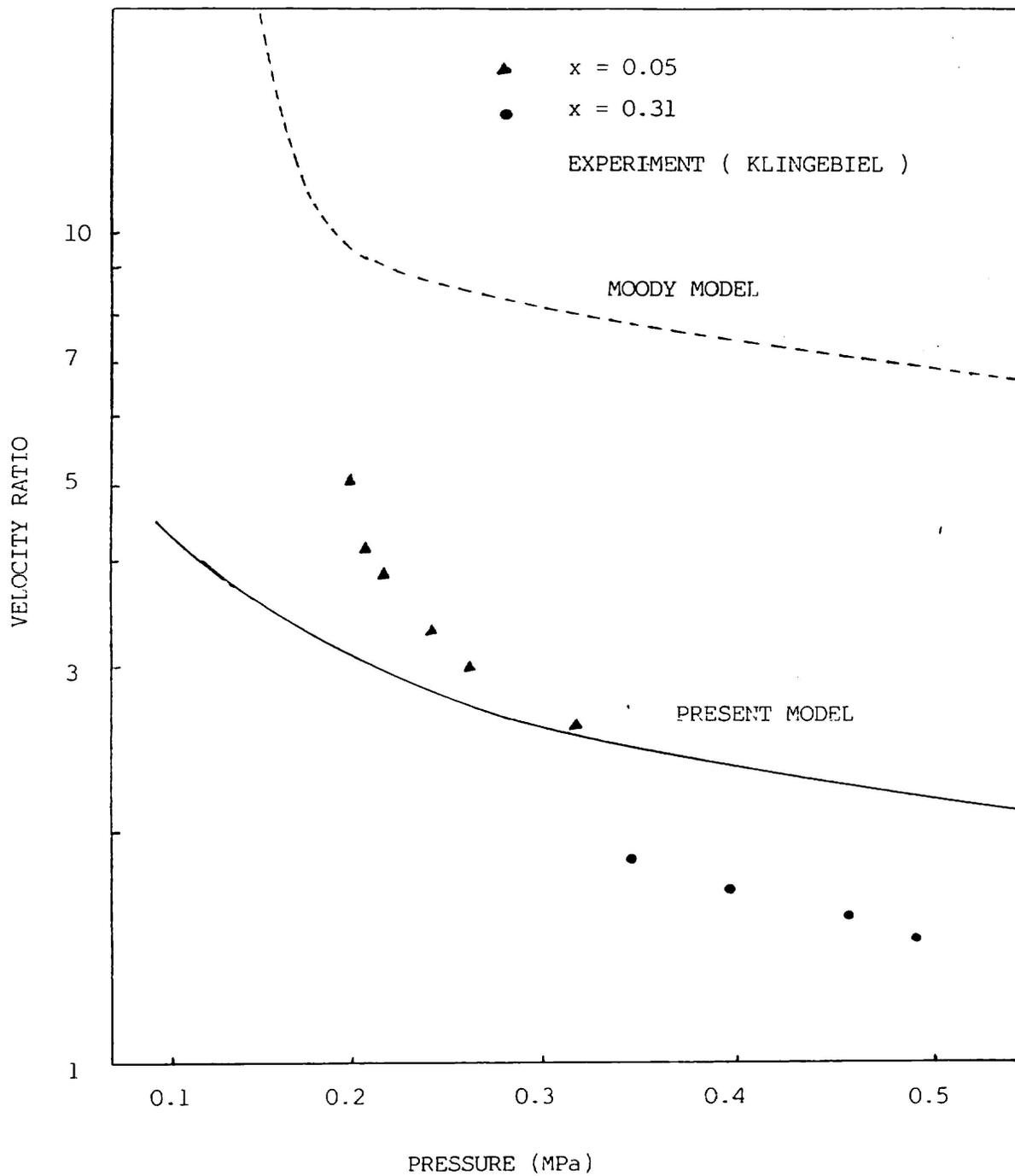
Figure 3. Comparison of theoretical and experimental slip ratios for steam water mixtures
