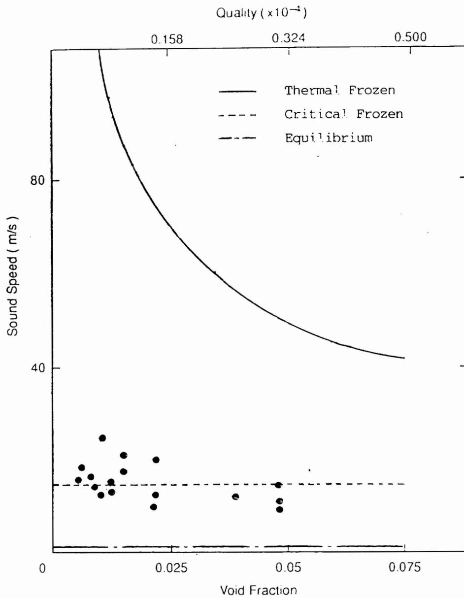
Figure 4. Comparison of sound speed with experimental data of Barclay et al. (  $p = 100$  kPa )
