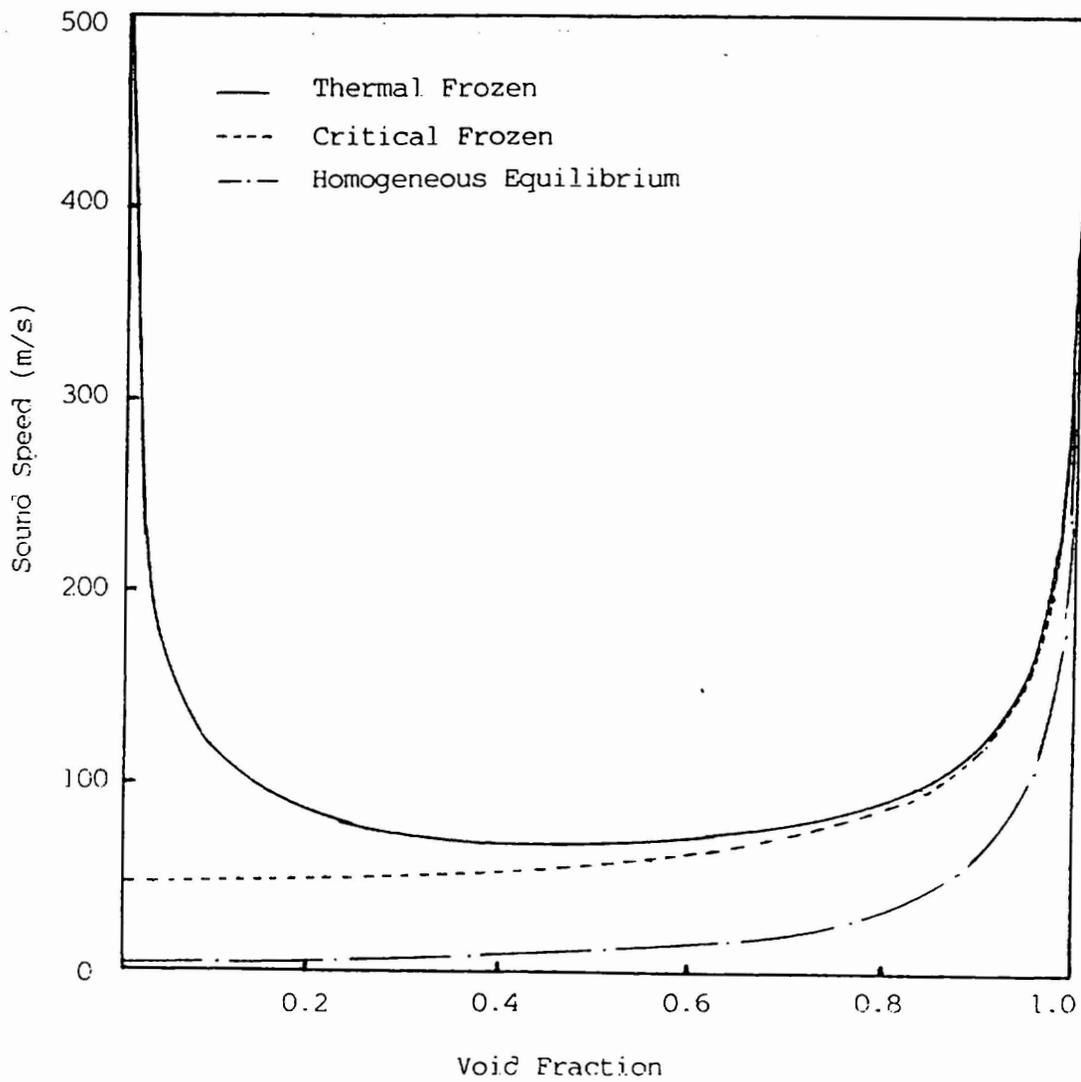
Figure 1. Comparison of the sound speeds of a homogeneous model at  $P = 1$  MPa of heavy water
