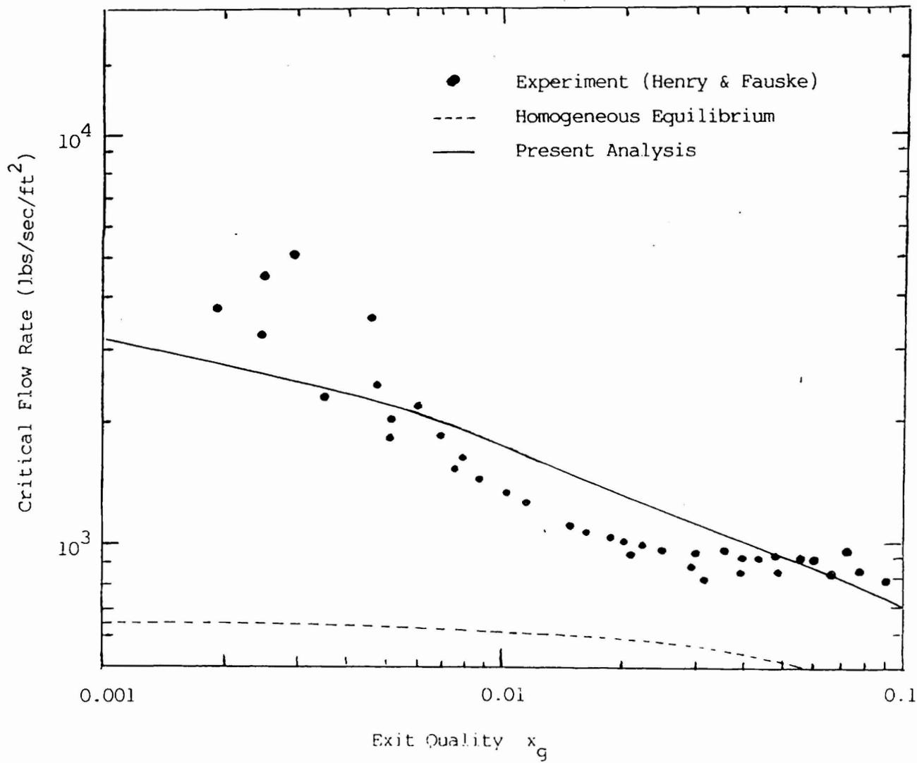
Figure 8. Comparison of predicted and experimental critical flow rates
