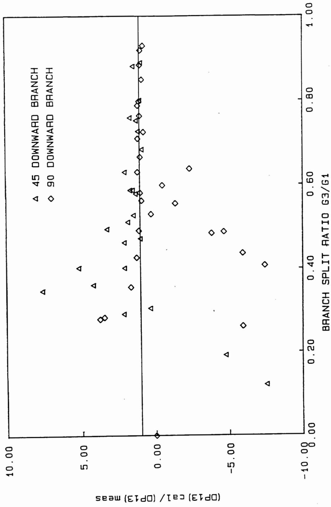
Fig.6. Comparison of branch pressure drops predicted by Saba & Lahey's homogeneous model with experimental measurement.
