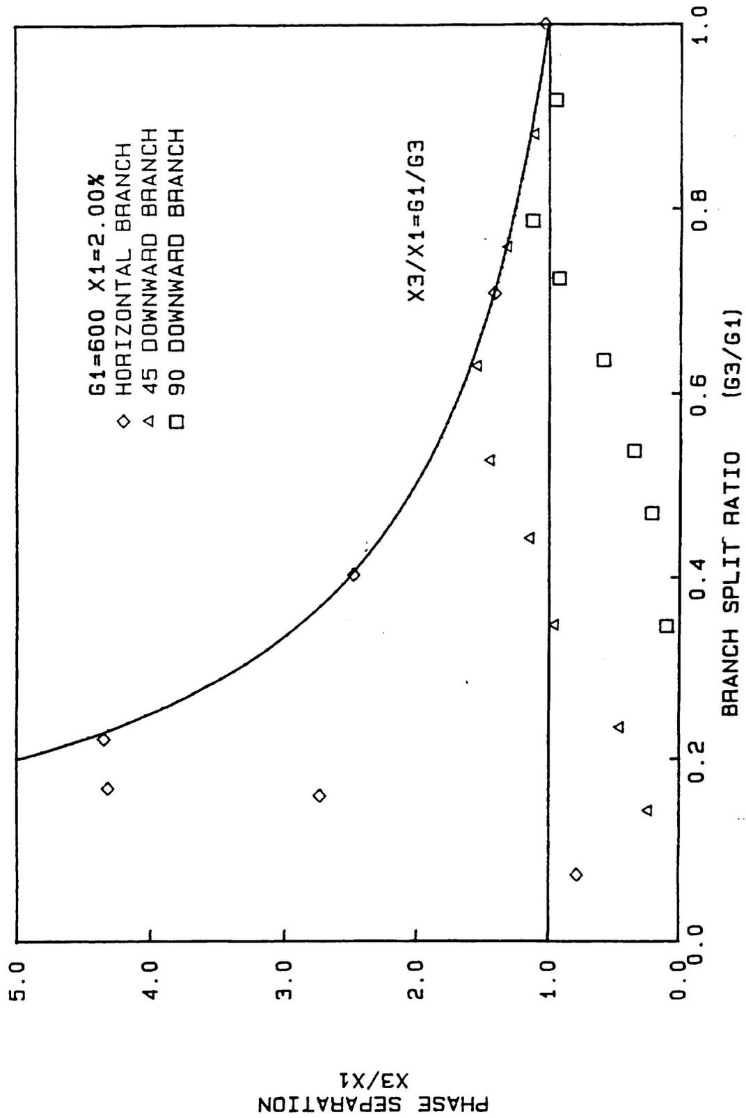
Fig.2C. Effect of branch orientation on phase separation.
