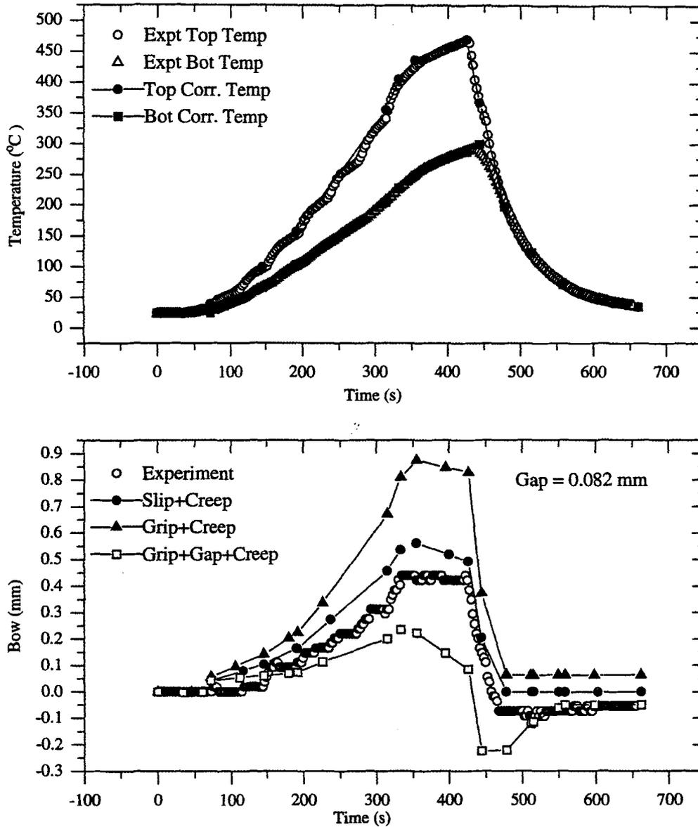
FIGURE 4: LINEARIZED TEMPERATURE-TIME CURVE (SOLID LINES) USED AS INPUT TO ABAQUS MODEL (TOP) AND A COMPARISON OF THE MODEL PREDICTIONS WITH THE MEASURED BOW FOR A BOW TEST WITH A LARGE DIAMETRAL GAP OF 0.082 mm
