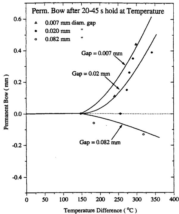
FIGURE 6: PERMANENT BOW AFTER 20-45 s HOLD AT TEMPERATURE AS A FUNCTION OF GAP SIZE
