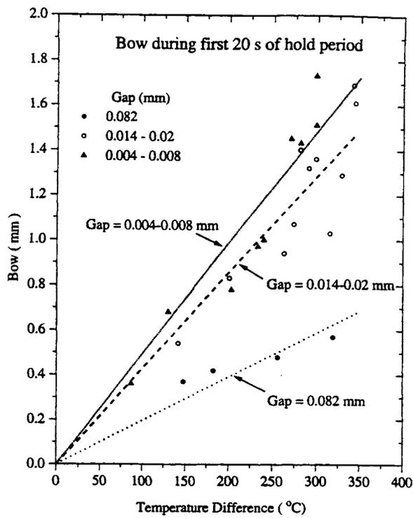
FIGURE 5: RELATIONSHIP BETWEEN AVERAGE TOP-TO-BOTTOM TEMPERATURE DIFFERENCE AND BOW DURING THE FIRST 20 s AT TEMPERATURE. THREE GROUPS WITH DIFFERENT DIAMETRAL GAPS ARE IDENTIFIED.
