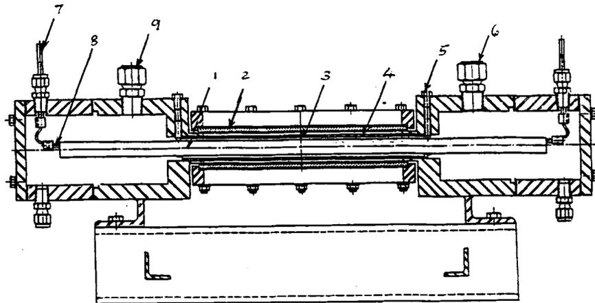
FIGURE 2: BOW TEST CHAMBER: (1 = FUEL ELEMENT SIMULATOR, 2 = QUARTZ WINDOW, 3 = OPENING FOR BOW MEASUREMENT, 4 = FLOW TUBE, 5 = SUPPORT PINS, 6 = He INLET, 7 = POWER CABLE, 8 = HEATER WIRE, 9 = HELIUM OUTLET)
