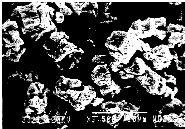
FIGURE 4: ELECTRON MICROGRAPH OF A POWDER PRODUCED FROM SPENT PWR FUEL USING THE OREOX PROCESS.
