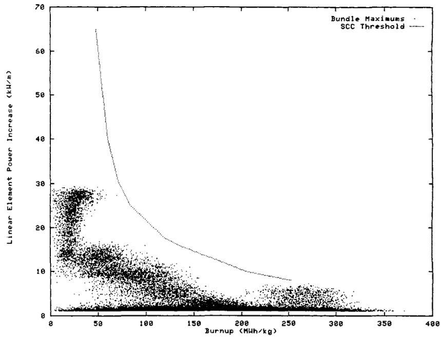
FIGURE 1. POWER BOOST ENVELOPE WITH STRESS-CORROSION CRACKING THRESHOLD
