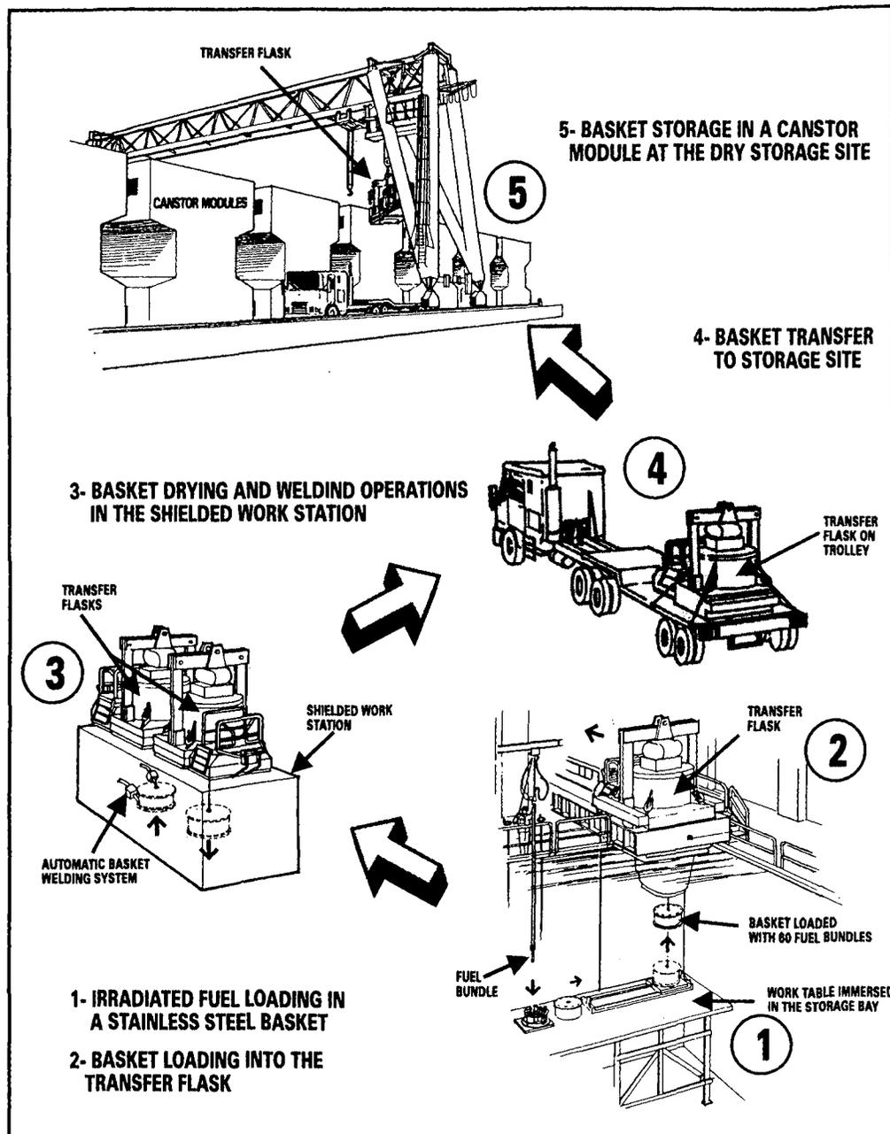
Figure 7 -Irradiated Fuel Dry Storage Sequence of Operations
