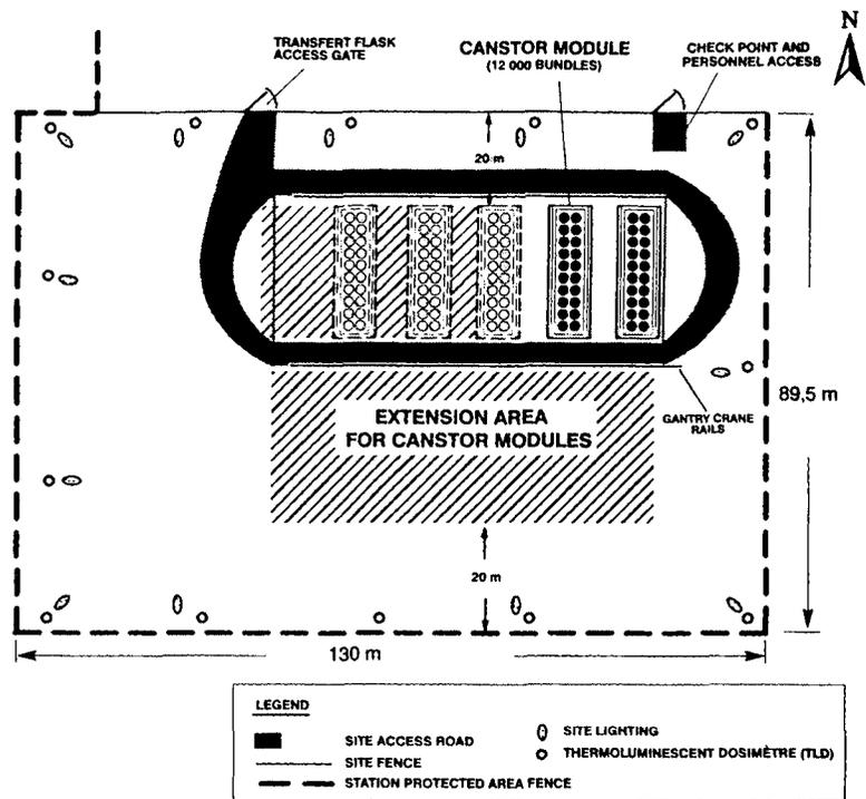
Figure 6 – Irradiated Fuel Dry Interim Storage Site
