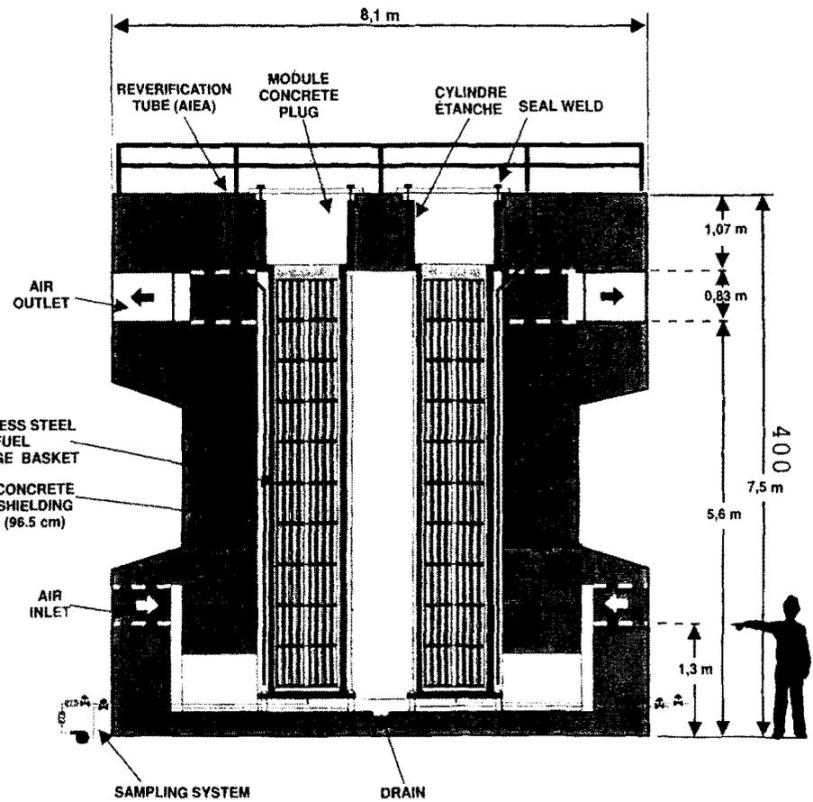
Figure 2 Section View of the CANSTOR Module
