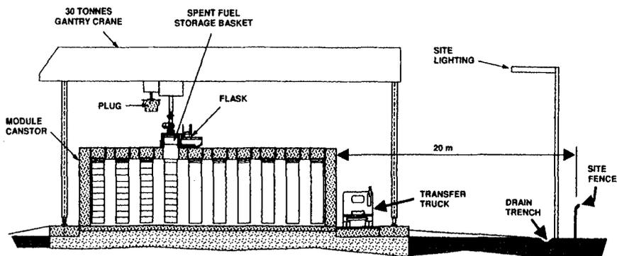
Figure 8 -Canstor Module Loading -Section View-
