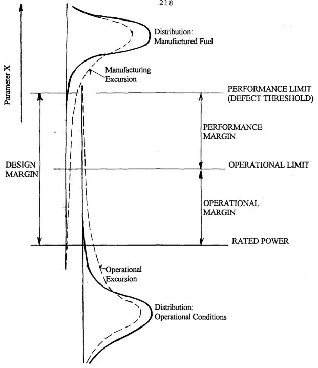
Figure 2 - Fuel Limits and Margins: Probability of Non-conformance and of Defects
