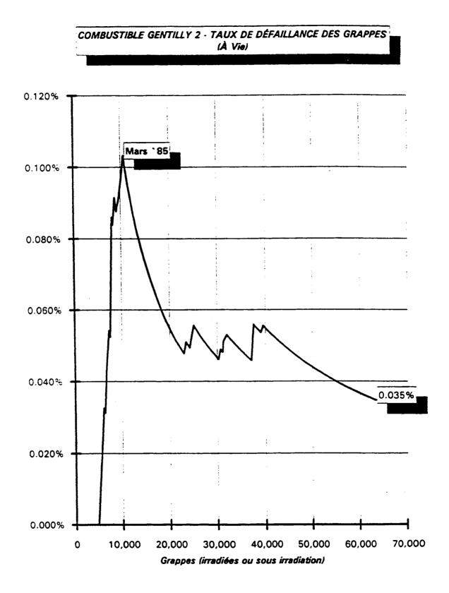
Figure 2 Gentilly-2 Fuel Defect Statistics
