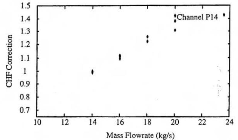
**Figure 4: CHF Correction for Channel P14**
